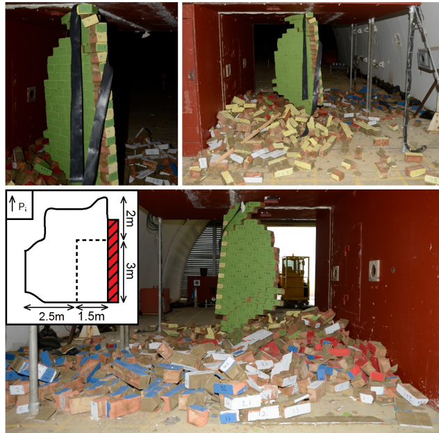
Figure 23: Debris distribution of structure BWL3C
