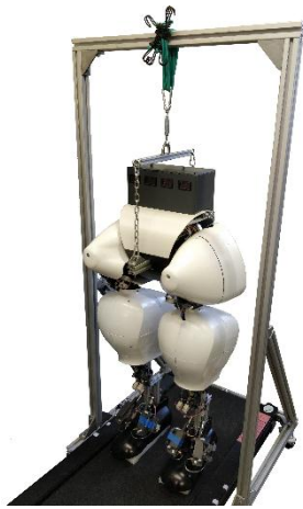
Figure 2. S.A.R.A.H. standing on a treadmill, supported by an elastic band.
