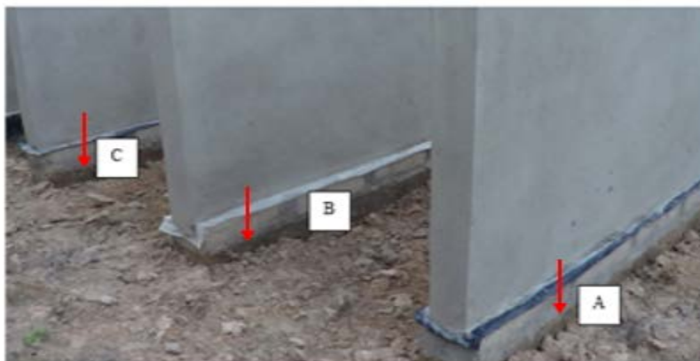
438 Fig 12 Water rise at the bases of the walls treated with three different DPCs - 0.15 mm thick (A), 439 0.12 mm thick (B) and 0.13 mm thick (C)
