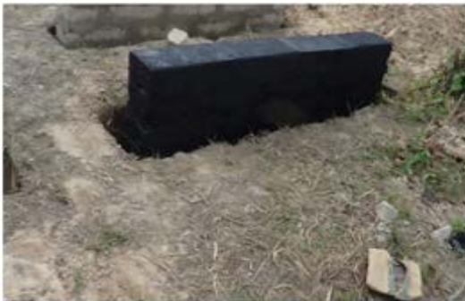
282 Fig 5 Photographs of the walls after the damp proof coatings 'A' (left) and 'B' (right) were 283 applied
