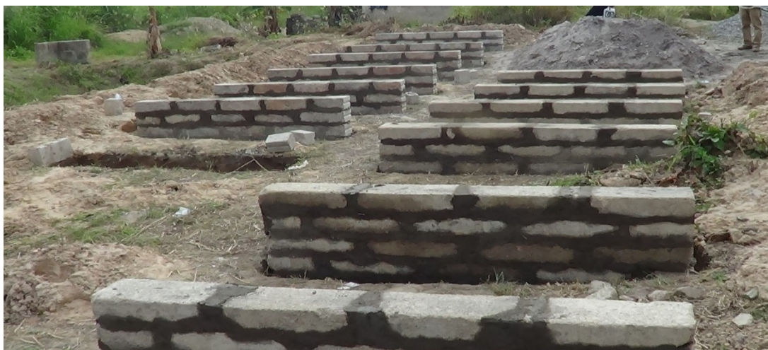
235 Fig 1 Photograph of test walls (extreme left are those constructed with SBs and extreme right are 236 those constructed with CBs) (Source: Agyekum et al. , 2016)
