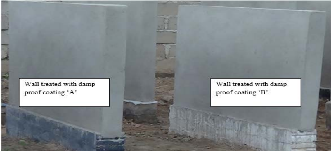
297 Fig 6 Photograph of test walls after they were treated with the damp proof coatings
