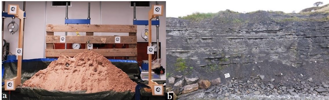
Figure 1: a) Lab experimentation: the slope was composed of sharp sand and was 1.5m long, 0.5m wide, 0.5m high and with a gradient of 60°. b) A section (25x20m) of an unstable sea cliff was selected for field verification.
