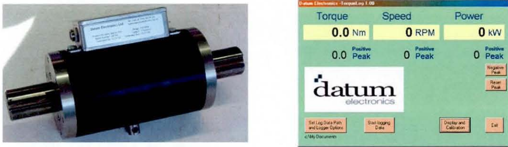
Figure 5.24 Torque Measurements using Datum Torque Transducer and Torque Log
