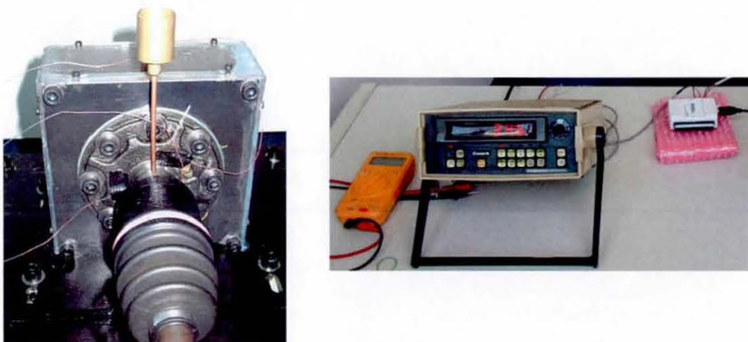
Figure 5.22 Temperature Measurements using Comark Microprocessor Thermometer
