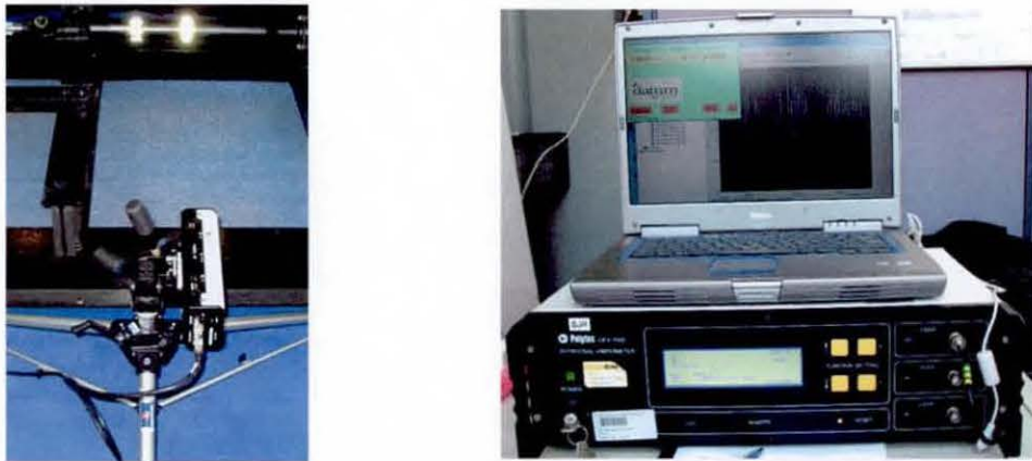
Figure 5.23 Rotational Speed Measurements using Laser Rotational Vibrometer
