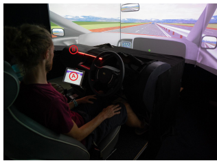
Figure 2: Apparatus: (A) tablet with fixation point attached to the centre; (B) peripheral light strip
