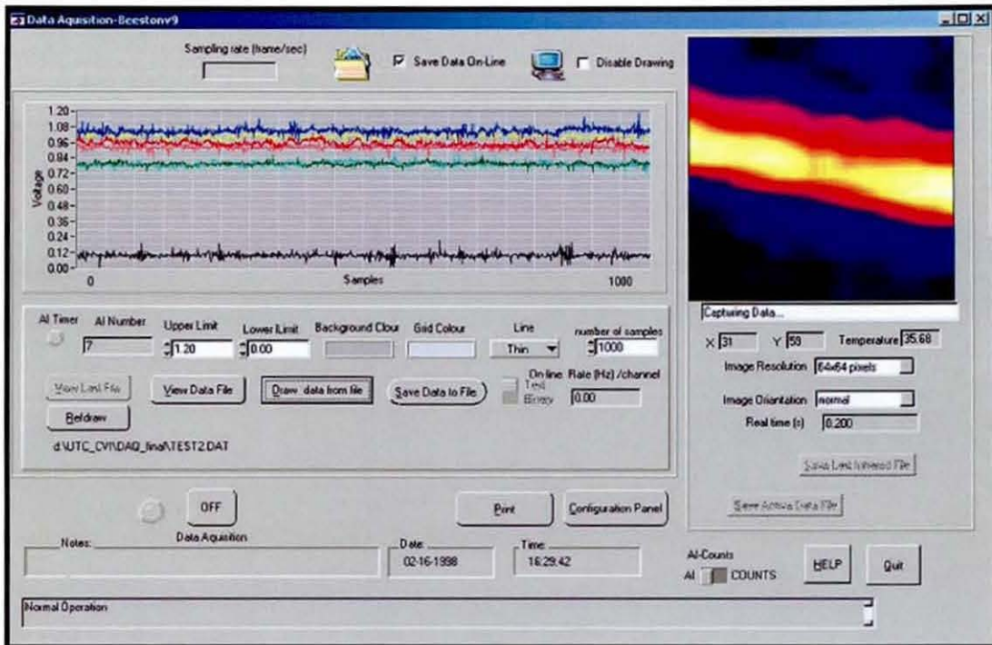
Figure 5.8. Thermography Condition Monitoring GUI. Screen 1, Al-Habaibeh et al. [2003].
