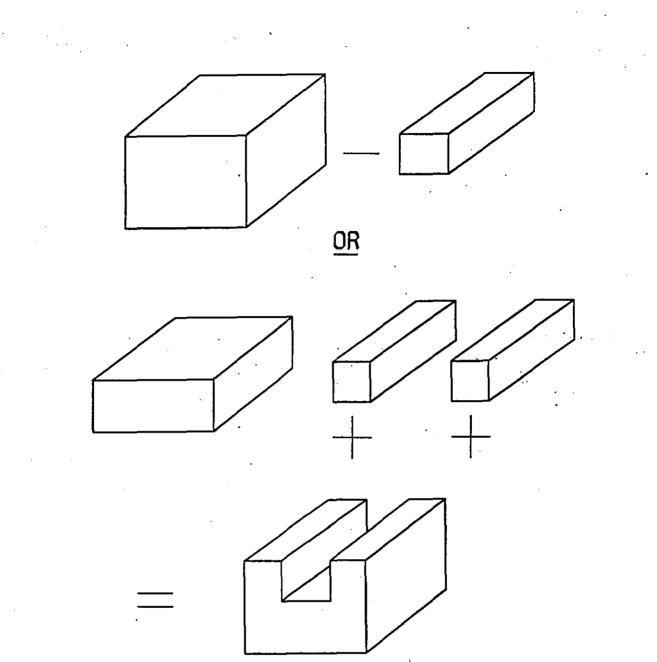
Figure 3.8 : Alternative Way in Creating a Slot.
