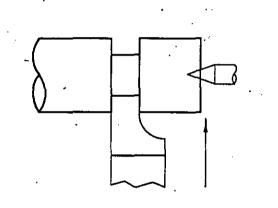
Figure 5.8 : Undercutting Operation.
