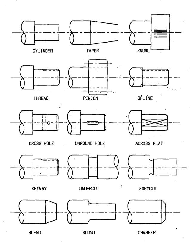
Figure 4.1 : Manufacturing Features of Rotational Component.
