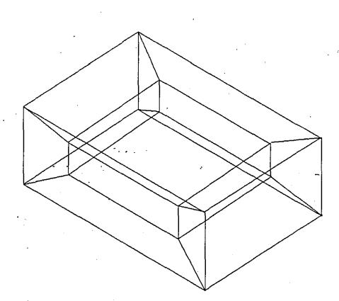
Figure 3.2 : Wire-Frame Modelling.
