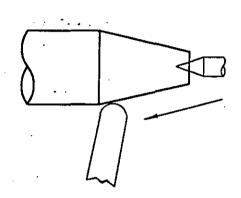
Figure 5.5 : Taper Turning or Tapering.
