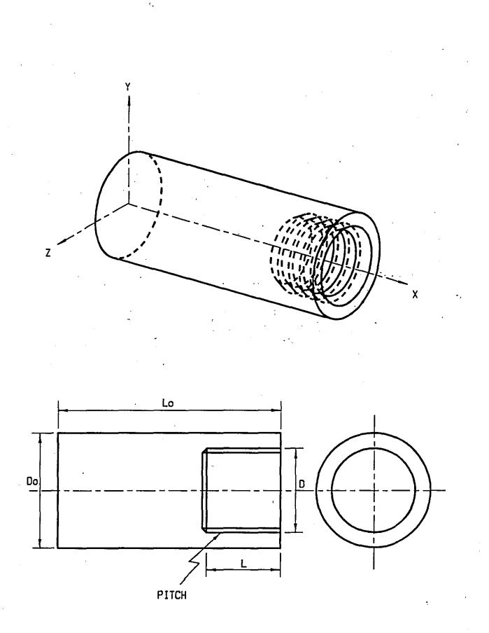
Figure 4.9 : Internal-Thread Feature.
