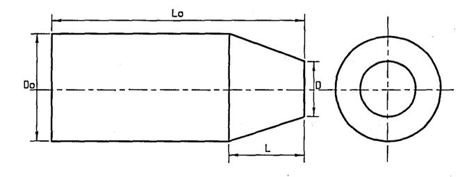
Figure 4.5 : External-Taper Feature.
