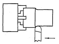
Figure 5.4 : Parallel or Straight Turning.
