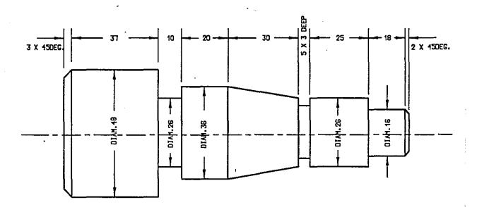
Figure 7.1 : Sample of External Features Component.
