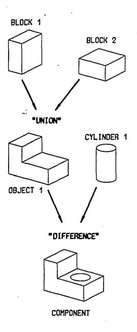
Figure 3.5 : The Tree Structure of the CSG Model.
