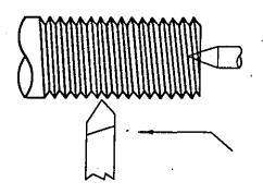
Figure 5.9 : External Threading Operation.
