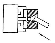
Figure 5.11 : Taper Boring Operation.
