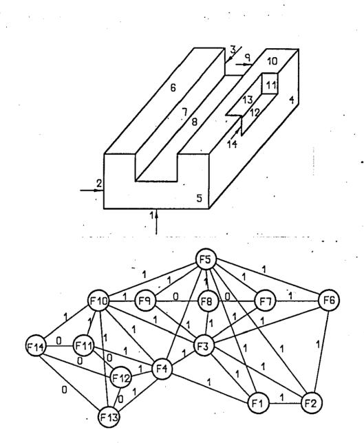
Figure 2.6 : An Example of AAG of a Component.
