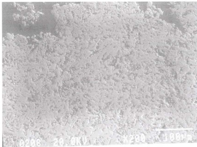
Figure 11 Tungsten powder after reduction of the W oxide ×200.
