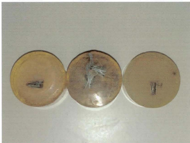
Figure 13 Swarf mounted and polished up to 6 microns
