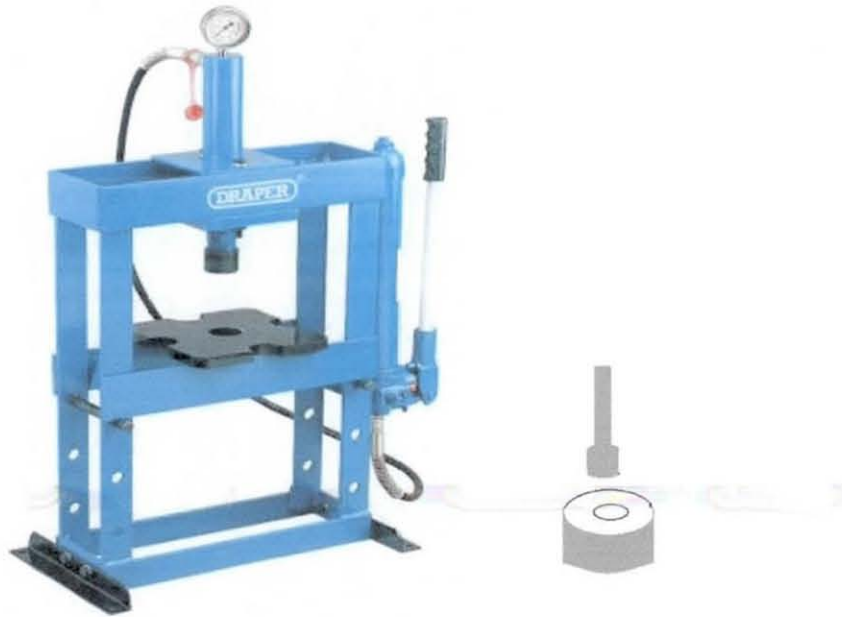
Figure 15 Draper press and 3.5 mm die
