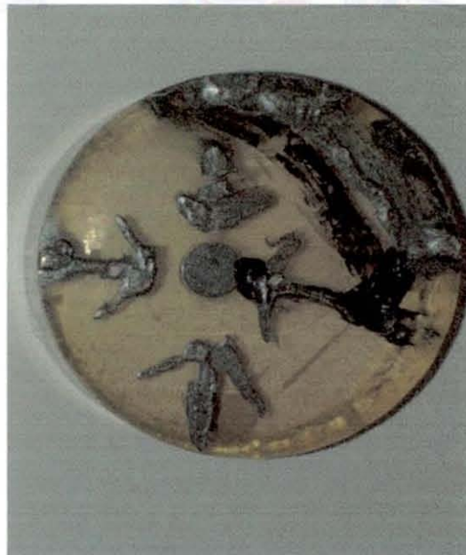
Figure 12 Tungsten pellet after pressing and sintering.
