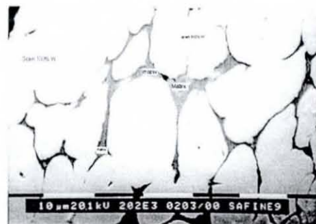
Fig. 1. Micrograph of the tungsten swarf material, showing tungsten grains embedded in a matrix material.
