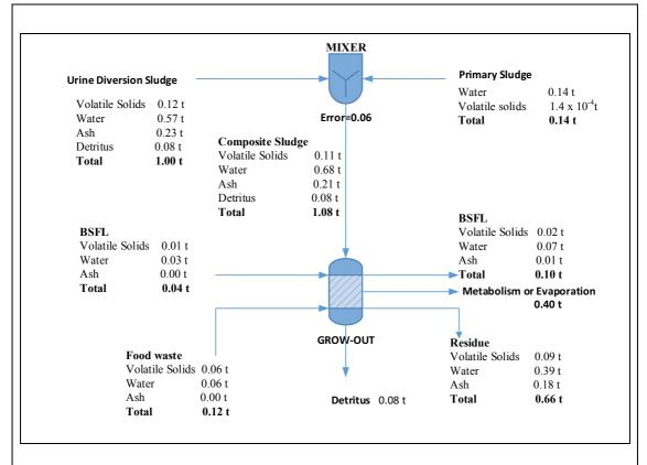
Figure 3. The Preliminary mass balance based on 1 tonne (wet basis) of UDT faecal sludge
