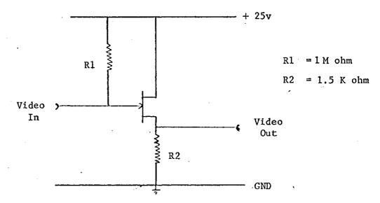
Figure A.12: Head amplifier for video signal.
