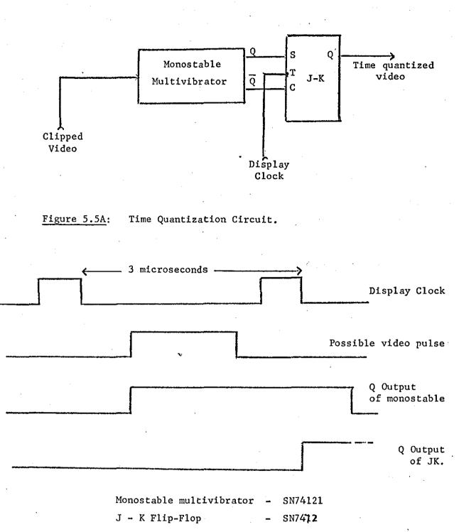
Figure 5.5B: Waveform diagram for Time Quantization process.
