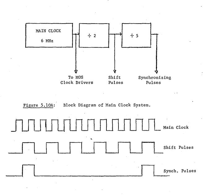
Figure 5.10B: Waveform Diagram of Clock System.
