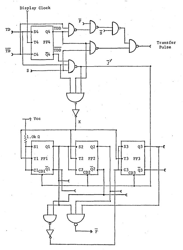
FF1, FF2, FF3, FF4 - TTL Master-Slave Flip-Flop SN7472
