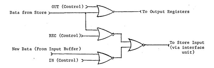
Figure 5.11C: Steering Circuit.
