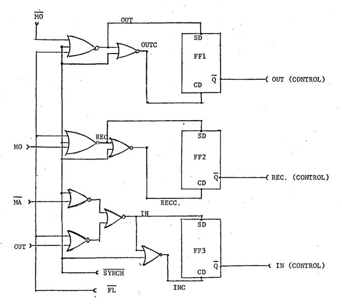
Figure 5.11B: Implementation of Input-Output Control Circuits.
