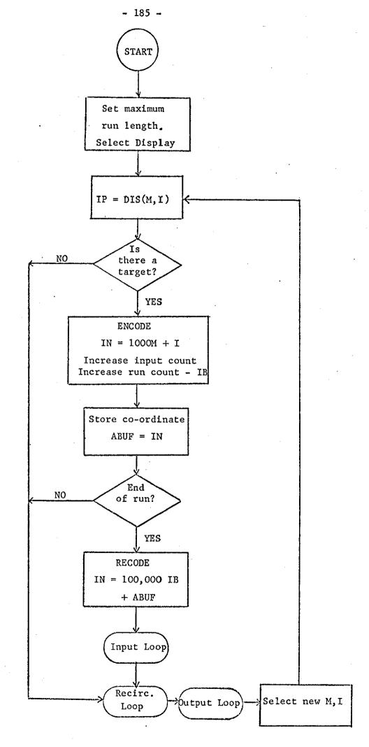
Figure A.8: Run Length Coding using Method 1.
