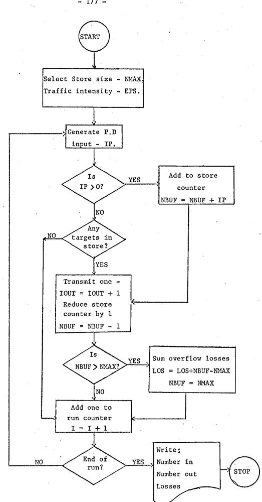
Simulation of step-down store with Poisson input. Figure A.3:
