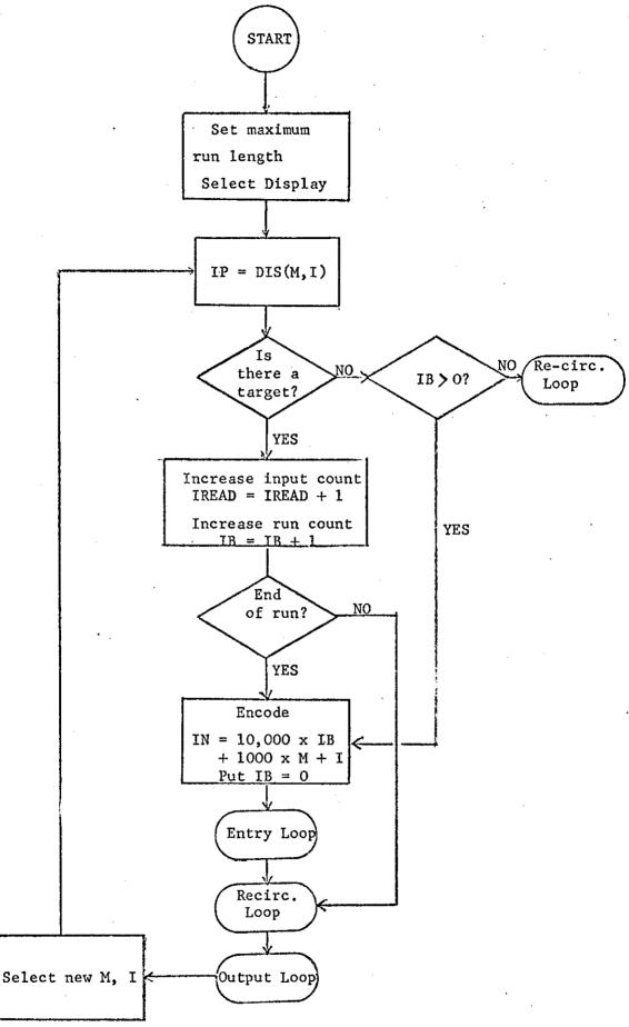
Figure A.9: Run Length Coding using Method 2.
