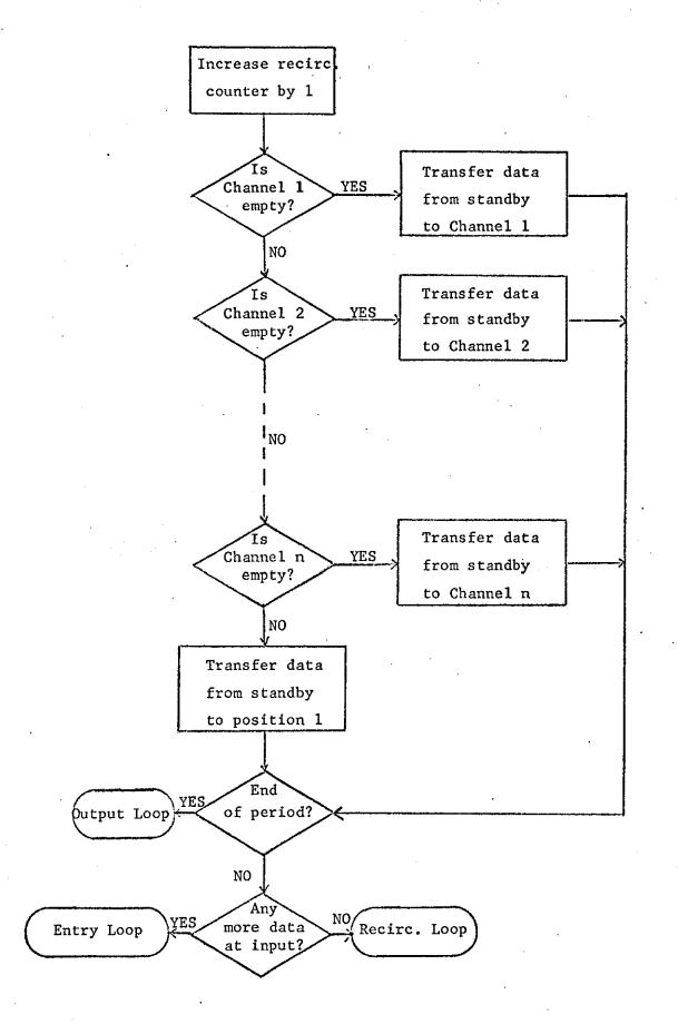
Figure A.6: Modifications to recirculation loop for multiple channels.
