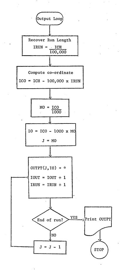
Figure A.10: Decoding process for run-coded inputs.
