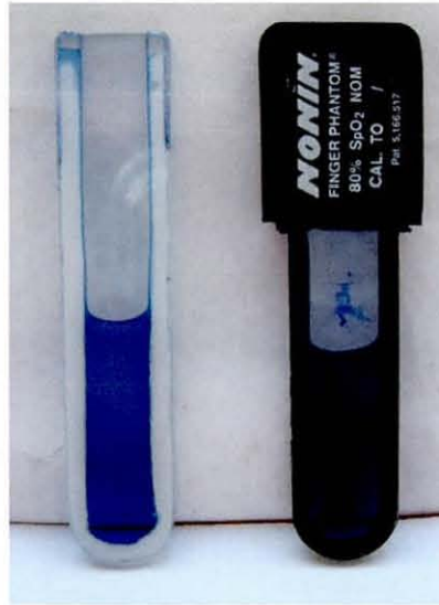
Figure 3.10 - Finger phantom constructed from microscope glass slides (left)
