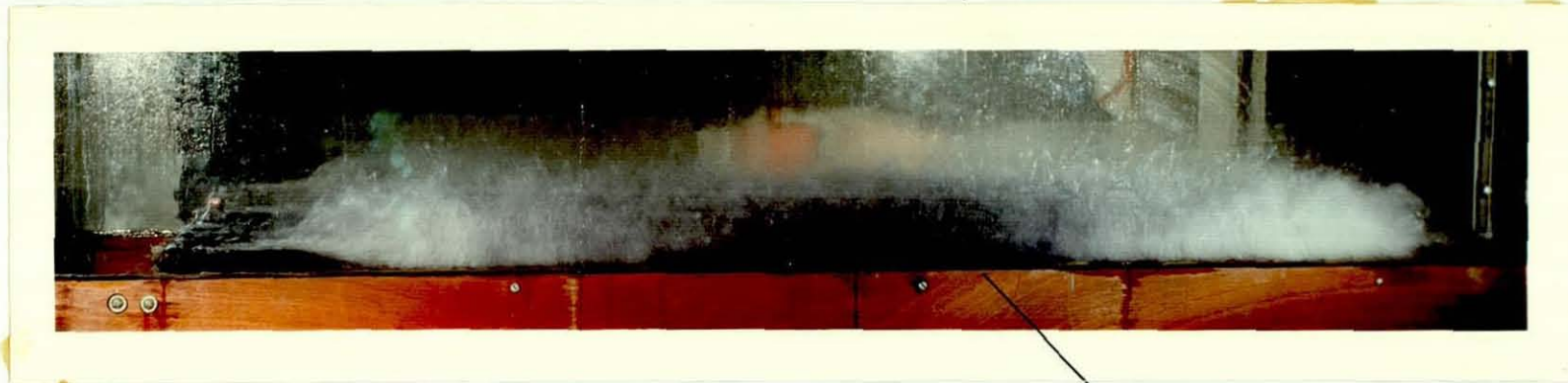
Photograph A. Taken 10 seconds after the injection. Injection point. The photograph shows the absence of perfect mixing and the presence of backmixing.
