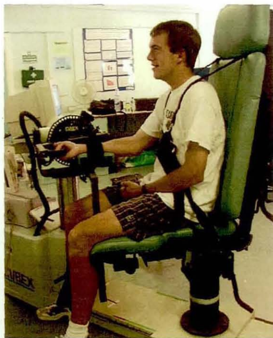
Figure 5.3. The subject and the dynamometer set-up for wrist flexion.
