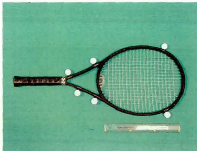
Figure 4.2. Head LM8 tennis racket with retro-reflective markers.
