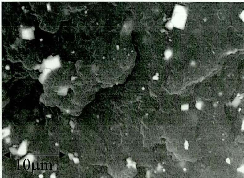
Plate 4.20, Back Scattered SEM Image of HIPS Containing 12wt.% DBDPO and 4wt.% RS Compounded Using A Twin Screw Extruder
