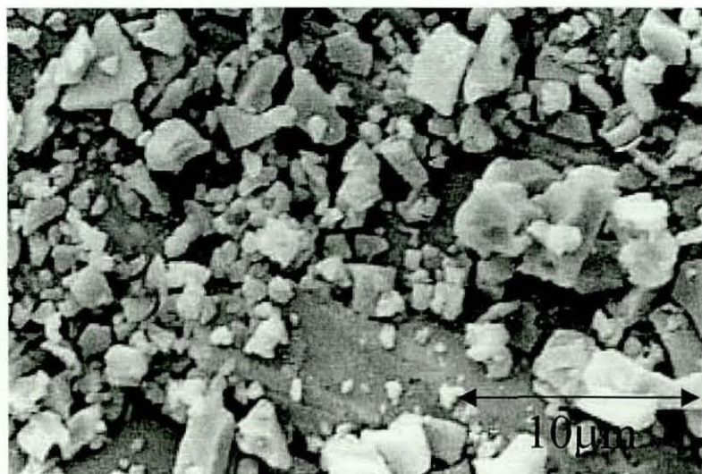
Plate 4.7, SEM Image of BC52 Grade of Tetrabromobisphenol A
