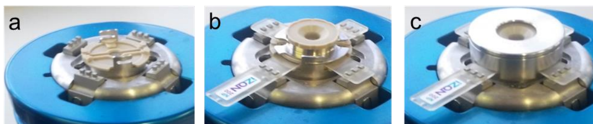
Figure 2.3 a) The lower fluid cell and teeth for mounting the nanopore. b) The pore is placed onto the teeth and upper fluid cell twisted into place. c) Faraday places over the fluid cell.
