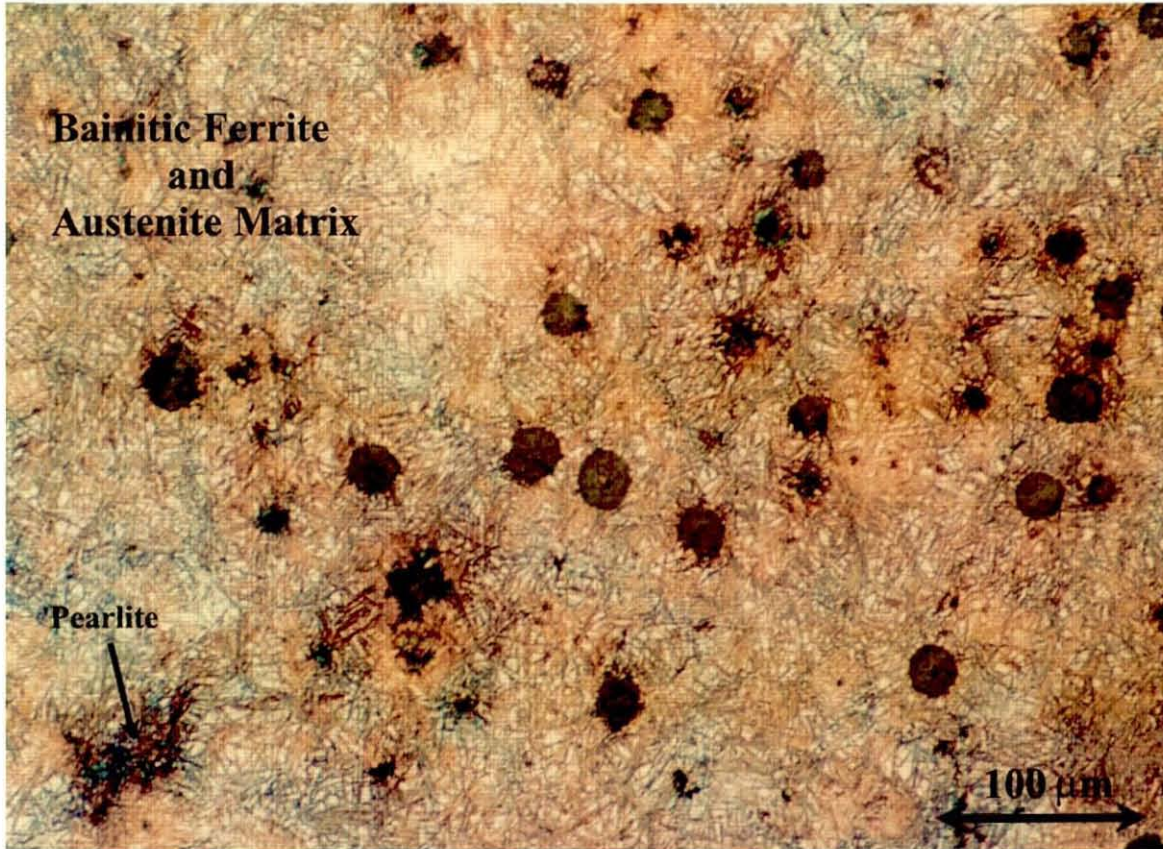
Figure 10.39. Optical micrograph of alloy 5f after austempering.
