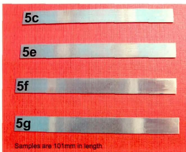
Figure 10.30. Oxide films on alloy 5 samples.
