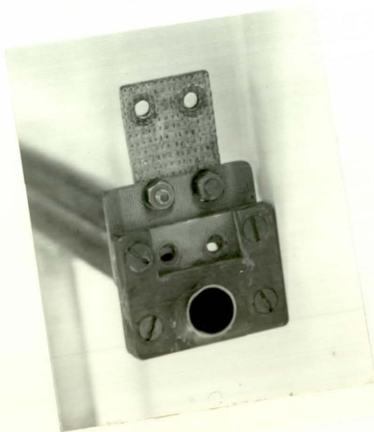
Fig. 13-6 (b) Detail of end fixing of Yoke for tube Assembly
