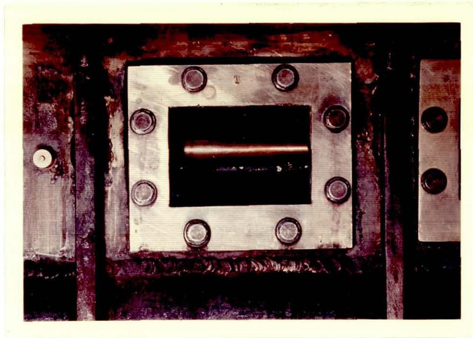
Fig. 16-4 Filmwise Condensation on a Horizontal Tube in the presence of Mechanical Oscillation (20 c/s, a = 0.17 ins) Tube at Maximum Positive Displacement
