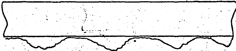
Fig. 2c Filmwise Condensation in the presence of tube vibration (20 c/s a_{\max} = 0.17 ins). Tube at maximum downward displacement
