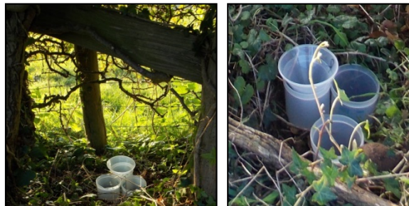
Figure 5.13: Throughfall buckets in triplets underneath the hedgerow.
