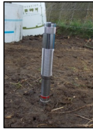
Figure 3.21: Pocket penetrometer in use at the Sheep Tree Shelter.
