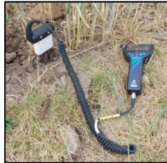
Figure 5.18: The HydroSense II probe in use at site.
