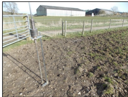
Figure 3.18: The dynamic cone penetrometer and in use at Horse Field Gate.
