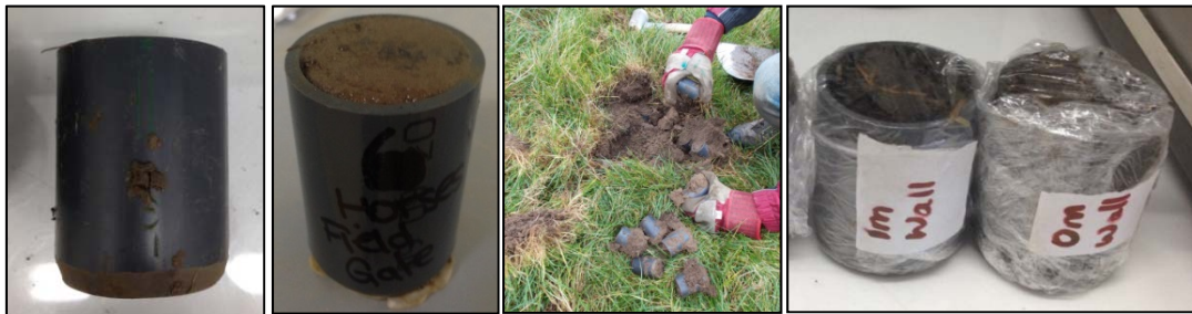
Figure 3.16: Core cutters used to collect soil samples from field sites.
