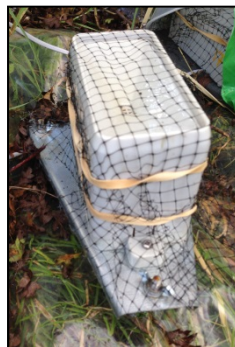
Figure 5.12: A throughfall gauge installed at site.
