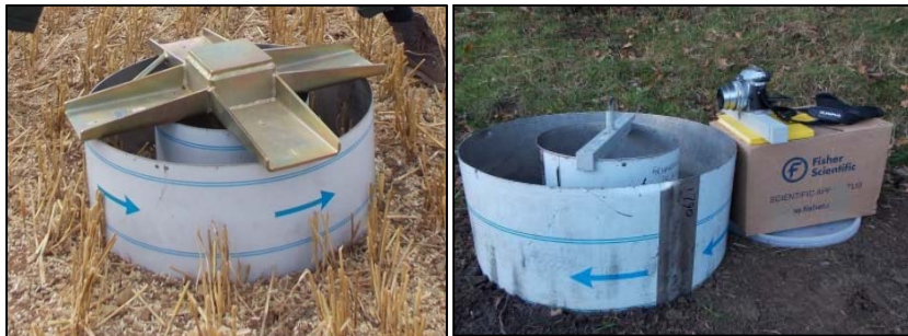
Figure 3.22: Installation and set-up of infiltrometer at Horse Tree Shelter.
