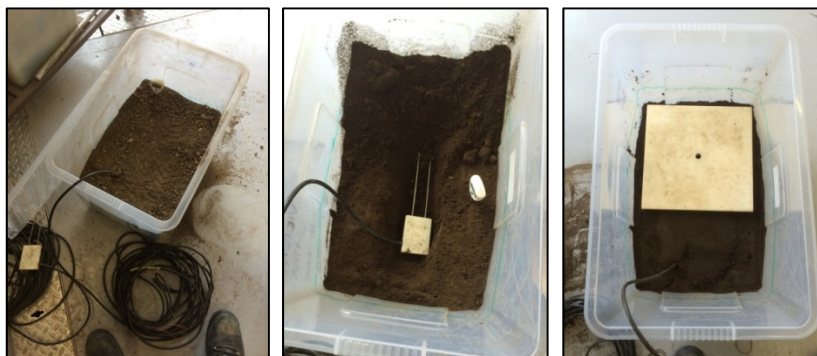
Figure 5.22: Calibration box, TDR probe in the box and compaction plate.
