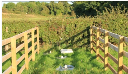
Figure 5.10: TBR gauges installed on west-side of the Hedgerow.
