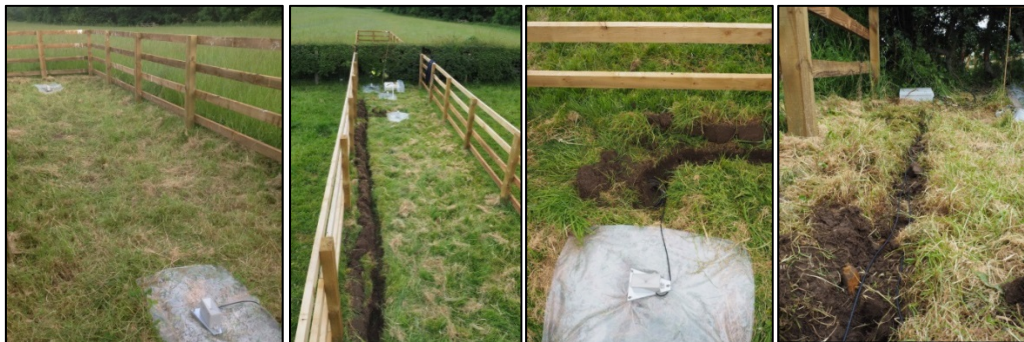
Figure 5.9: TBR gauge installation at Hedgerow Site.
