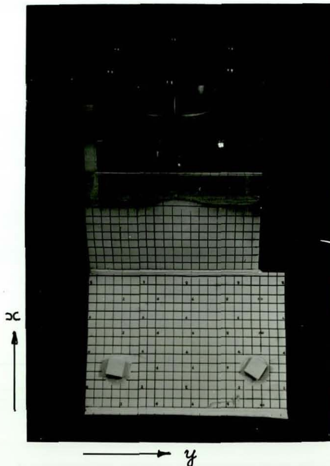
Fig. 5.2 The side wall on which measurements of strain were made
