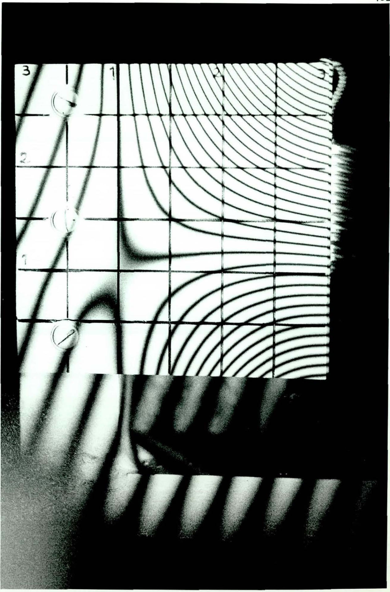
Fig. 4.11 Interferogram due to the combined effects of an incremental load and a small rotation of the beam directing mirror
