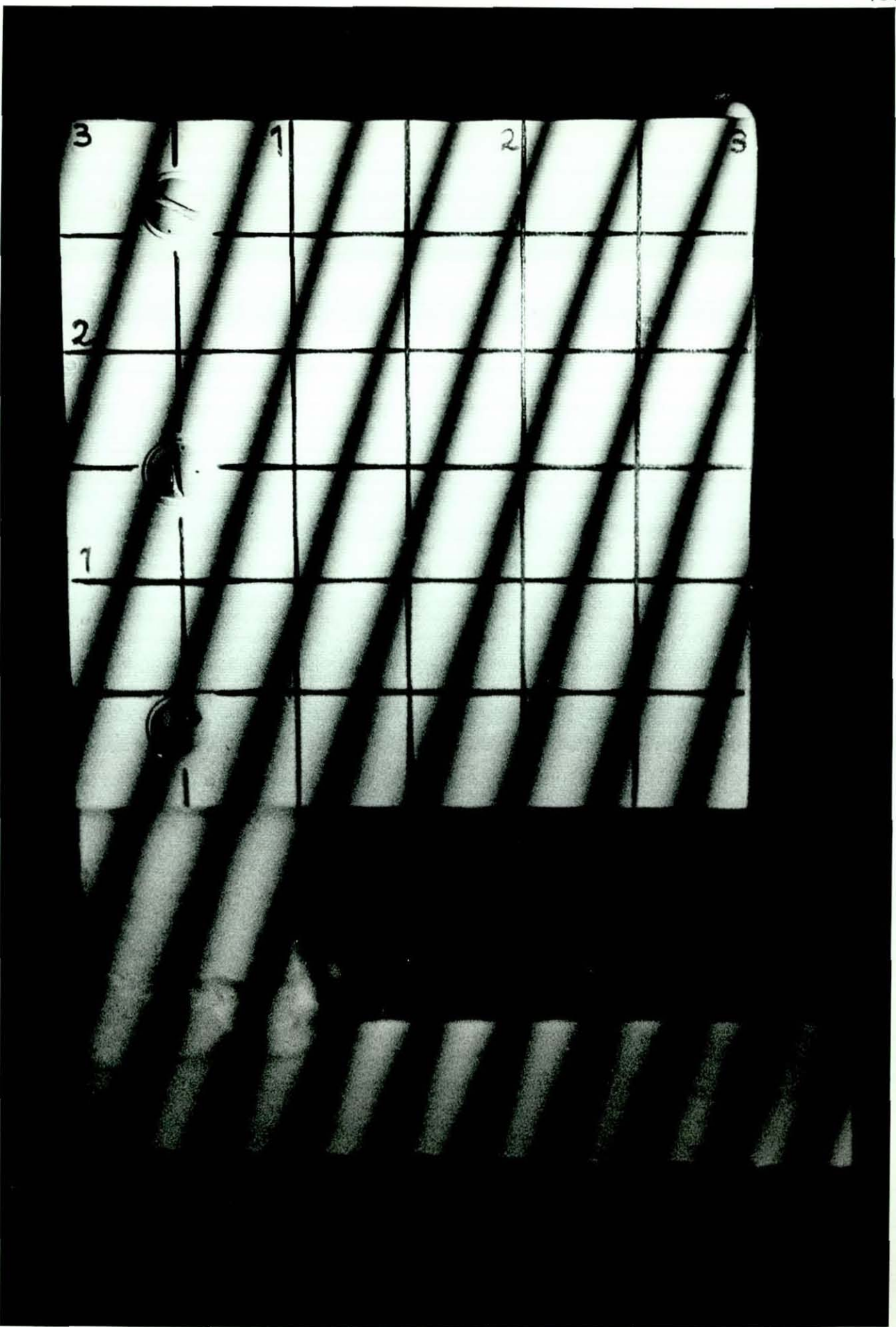
Fig. 4.12. Interferogram over the plate due to a small rotation of the mirror directing the object illumination beam
