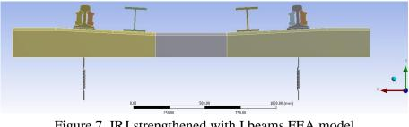
Figure 7. IRJ strengthened with I beams FEA model
