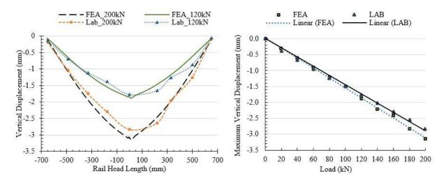
Figure 4.42 Comparison between FEA calculated and measured by dial gauges deflection results of the 3-point bend test
