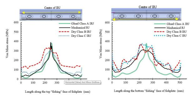
Figure 24. Equivalent (von-Mises) stress plots of the centre of top and bottom fishing surface of the fishplate for various rail joint types
