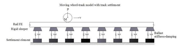
Figure 2.5 Moving wheel-track settlement model produced from Dahlberg (2001)
