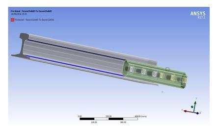
Figure 8. Frictional contact between rail and fully encapsulated fishplate
