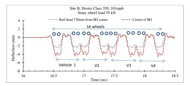
Figure 4.8 Deflection time histories under the passage of four-vehicle Desiro at 101mph.
