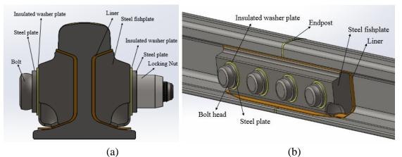
Figure 1. (a) cross and (b) front section of a glued Class A IRJ
