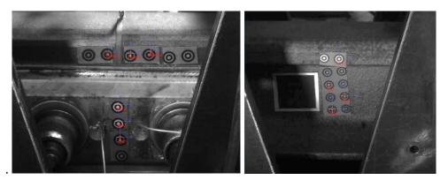
Figure 4.2 Video images showing measurement positions of (i) IRJ rail head and fishplate web and (ii) plain rail head and web during the 4-point bend test.
