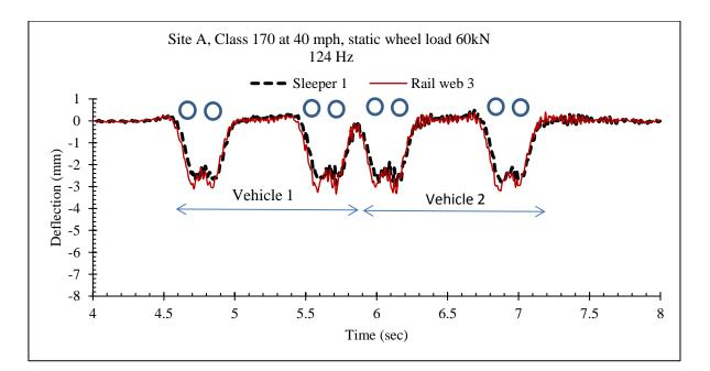
Figure 4.5 Rail and sleeper deflection at Site A under the passage of Class 170 at 40 mph.
