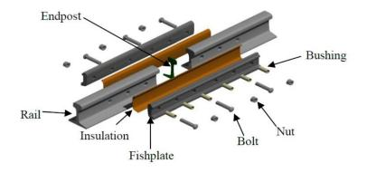
Figure 2.9 IRJ assembly (reproduced from Paper 3)
