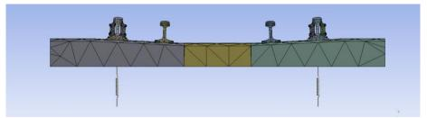
Figure 6. IRJ strengthened with strap rails FEA model
