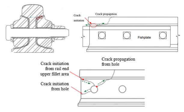
Figure 4.38 Potential fatigue failure modes amended from RAIB (2014)
