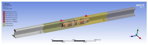
Figure 16. FEA model of 4- point bend configuration
