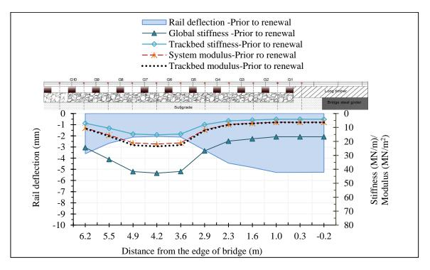
Figure 4.17 Deflection and stiffness properties along the transition zone –Phase I.
