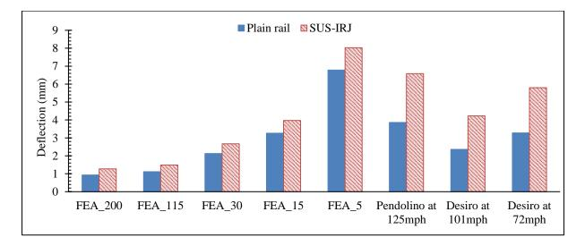
Figure 12. Comparison between FEA models and field deflection data for plain rail and SUS-IRJ.
