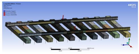
Figure 5. Geometry and meshing of the FEA model
