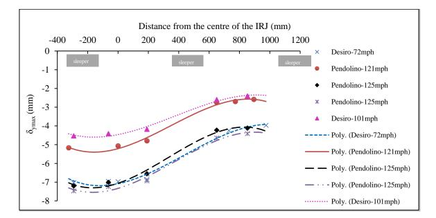
Figure 4 Maximum displacements of rail head at various distances from the centre of the IRJ.
