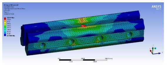
Figure 21. Equivalent (von Mises) stresses - Mechanical RJ
