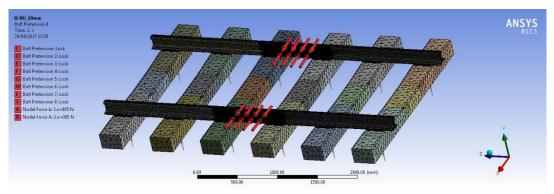
Figure 5. Model layout showing bolt preload and mesh
