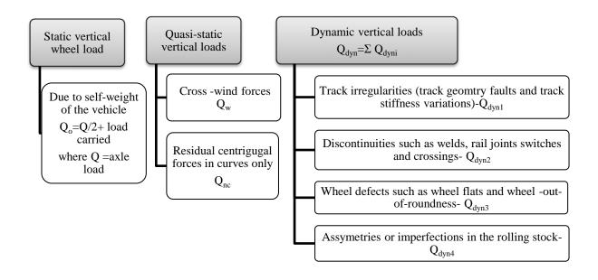
Figure 2.1 Classification of vertical loads, according to RSSB (2016)
