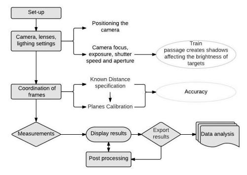
Figure 2 Set-up and measurement procedure
