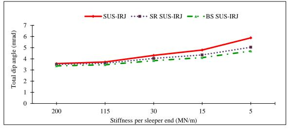
Figure 11. Effect of enhancement on total dip angle of suspended IRJs
