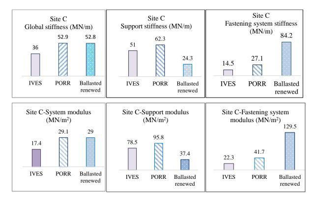
Figure 4.16 Stiffness characteristics calculated for Site C.
