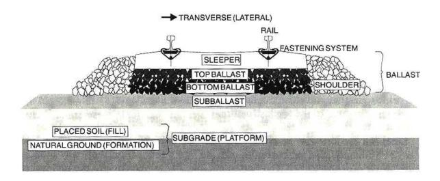
Figure 1.1 Conventional ballasted track structure from Selig and Waters (1994)
