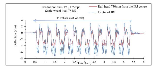
Figure 4.10 Deflection time history under the passage of 11-vehicle Pendolino at 125mph.
