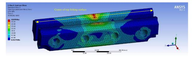
Figure 4.28 Equivalent (von Mises) stresses - Glued Class A IRJ- Load case 1
