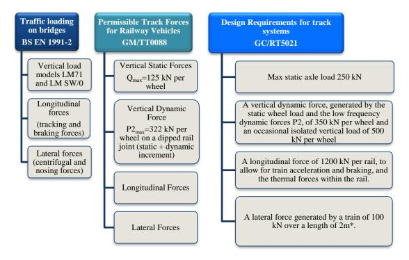
Figure 2.3 Design loading for track systems, according to RSSB (2016)
