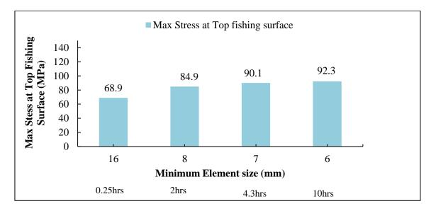
Figure 4.34 Mesh sensitivity study for Glued IRJ, Load case 2
