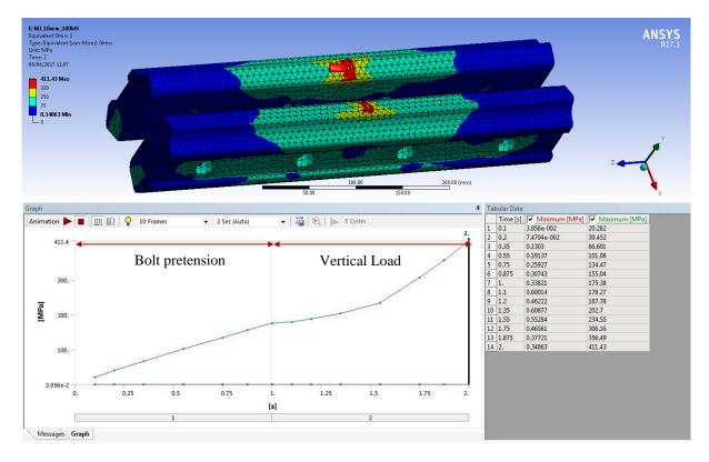
Figure 4.35 Equivalent (Von Mises) stresses  $\sigma_e$  - Mechanical RJ - 100kN preload - Load case 1 (i) stress contour (ii) magnitude during loading steps
