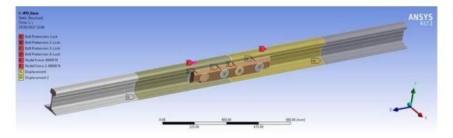
Figure 4.39 FE model of 4-point bend laboratory configuration
