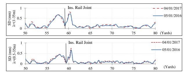
Figure 4.13 Vertical level from Site B [CGJ1], up fast [1100], 159 mile, left rail measured by HSTRC. Upper graph: wavelength band  $\lambda$ =[1, 35]m, lower graph:  $\lambda$ =[0.5, 35]m
