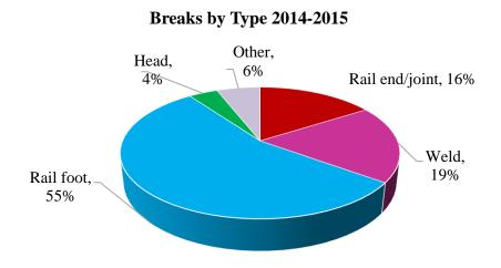
Figure 1.8 Rail breaks by type from Whitney (2015)
