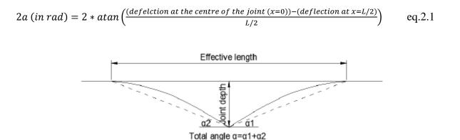
Figure 2.11 Idealised dip angle form, from Grossoni et al. (2014)
