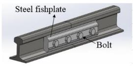
Figure 3. Tight mechanical rail joint
