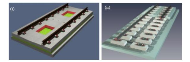
Figure 1.5 Examples of slab track (i) PORR-Austria and (ii) Rheda 2000- Germany adapted from Porrill (2015)
