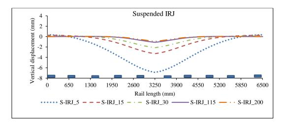
Figure 9. Deformation of suspended IRJ with stiffness variation.
