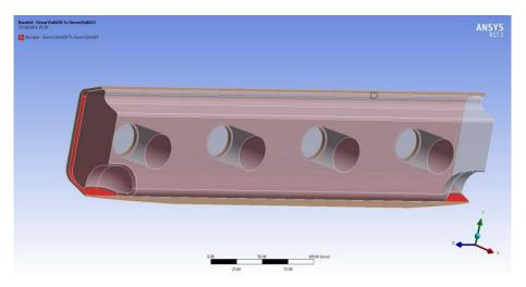
Figure 6. Bonded contact between (a) the rail and liner and (b) the fishplate and the liner to simulate glue.
