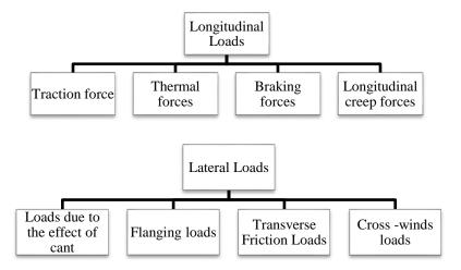
Figure 2.2 Track lateral and longitudinal loads, according to RSSB (2016)
