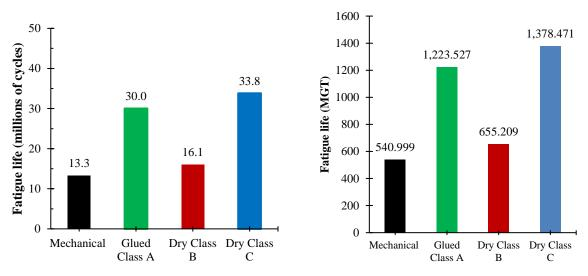
Figure 4. Calculated fatigue life of joints expressed in millions of cycles and in MGT.
