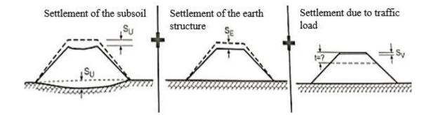
Figure 1.3 Reasons of track settlements adapted from Lichtberger (2005)
