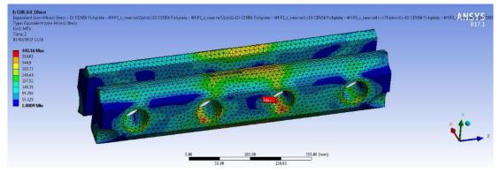
Figure 22. Equivalent (von Mises) stresses - Dry Class B IRJ
