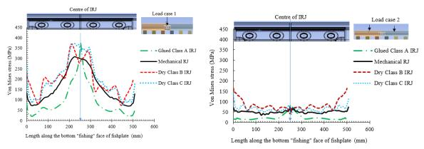
Figure 3. Equivalent (von-Mises) stress plots of the centre of bottom fishing surface of the fishplate for four rail joint types and two load cases.
