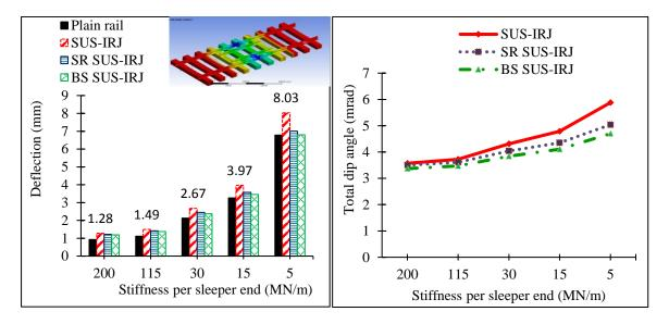
Figure 4.23 Effect of reinforcement on the deflection and dip angle of suspended IRJ for varying support stiffness from Paper 2
