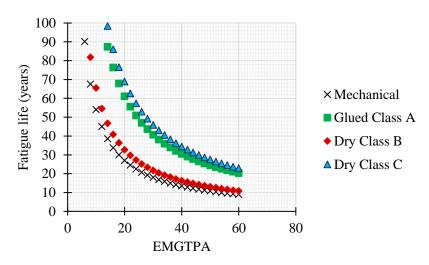
Figure 5. Calculated fatigue life of joints in years according EMGTPA
