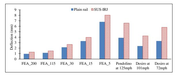
Figure 4.24 Comparison between numerical model and field deflection data for plain rail and SUS-IRJ from Paper 2
