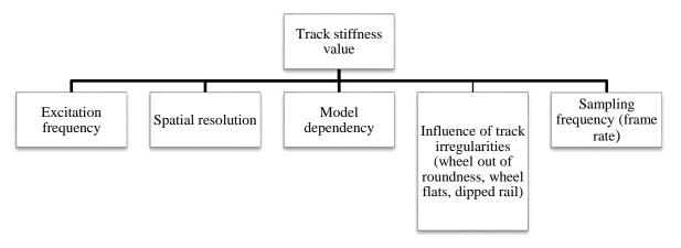
Figure 2.8 Factors affecting track stiffness sensitivity
