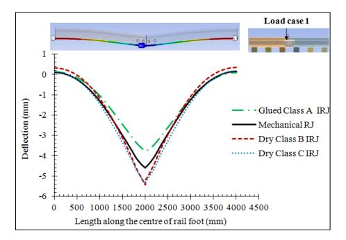
Figure 4.27 Deflection along the centre path of rail foot for four rail joint types
