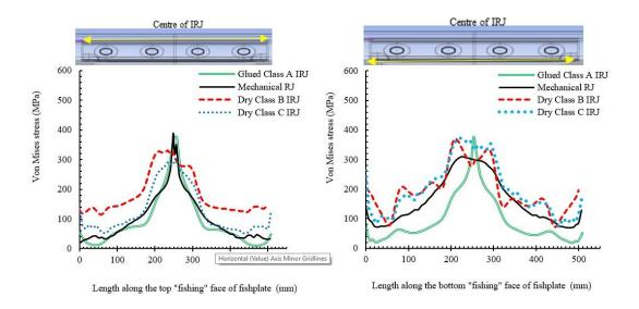
Figure 4.29 Equivalent (von Mises) stress plots of the centre of the top and bottom fishing surface of the fishplate for various RJ types.
