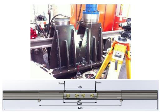
Figure 15. 4-point bend configuration
