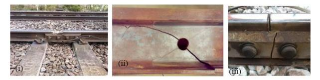
Figure 1.9 Examples of rail joint damage mechanisms from Whitney (2013) (i) broken rail head, (ii) cracks initiated from rail bolt hole and on the underside of the rail head and (iii) broken fishplate
