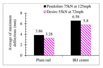
Figure 4.11 Comparison between IRJ and plain rail deflection for different trains and speeds.
