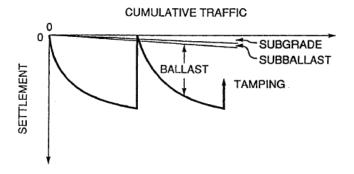
Figure 1.4 Substructure contributions to settlement from Selig and Waters (1994)
