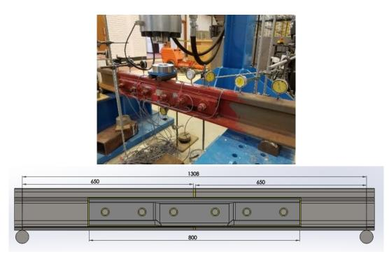
Figure 11. (a) Laboratory 3-point bend test showing set-up and position of dial gauges (b) Geometry of the 3-point bend configuration
