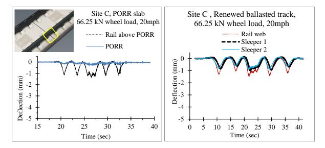
Figure 4.15 Deflections of PORR slab and renewed ballasted track at Site C.
