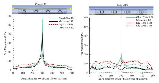
Figure 4.30 Equivalent (von Mises) stress plots of the rail head and foot fishing surfaces for various RJ types.
