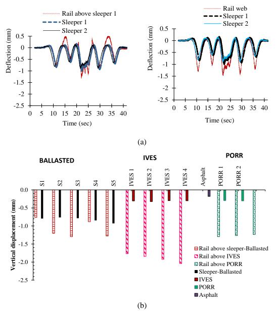
Figure 3. (a) Time-deflection plots of IVES, PORR and ballasted track under low speed train passage (b) comparison among maximum deflections.
