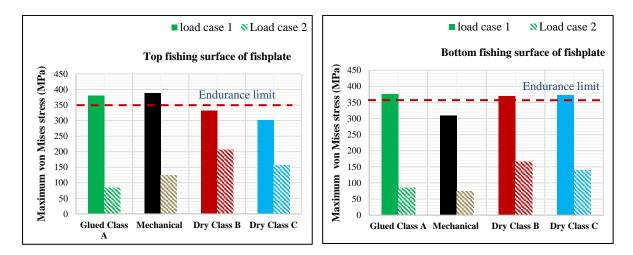
Figure 4.32 Maximum von Mises stress found in the fishing surfaces of the fishplates
