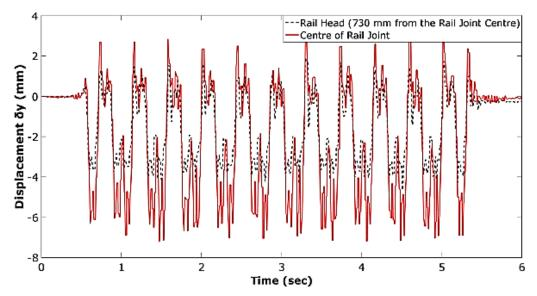
Figure 3. Displacement –time history for rail joint and plain rail during the passage of a Pendolino Class 390 train (125 mph)
