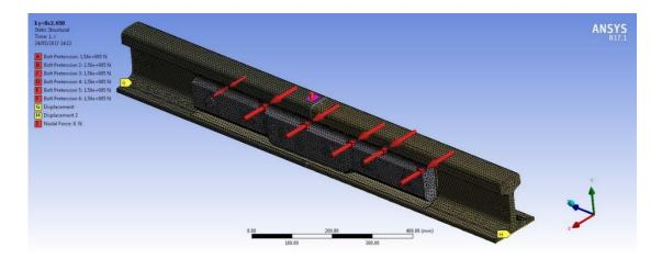
Figure 4.41 FE model (showing mesh, loading and boundary conditions) of the 3-point bend laboratory configuration
