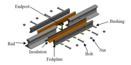
Figure 1. View of IRJ assembly (amended from [1])
