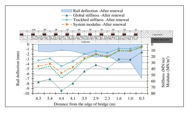
Figure 4.18 Deflection and stiffness properties along the transition zone -Phase II.
