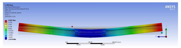
Figure 17. Vertical displacement of glued IRJ in a four-point bend FEA-load case 160 kN.
