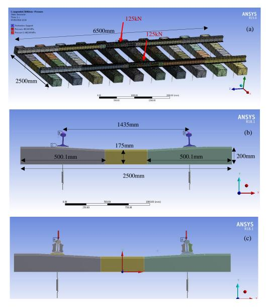
Figure 4.21 (a) Model layout and side view of (b) plain track model (c) suspended IRJ model amended from Paper 2
