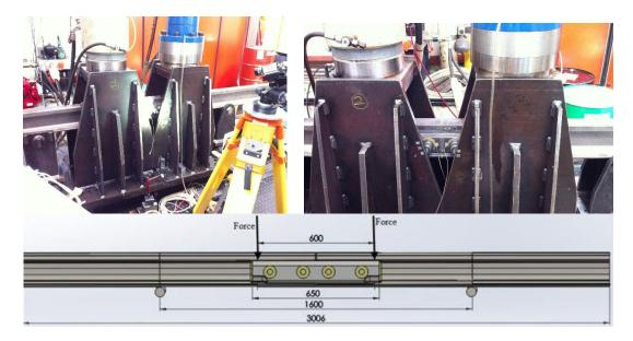
Figure 4.1 Four-point bending test configuration.
