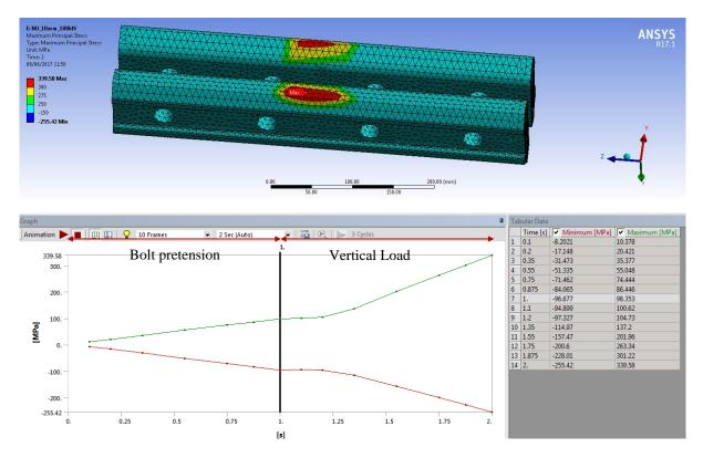
Figure 4.36 Maximum principal stresses  $\sigma_1$  - Mechanical - 100kN preload - Load case 1 – (i) stress contour (Bottom fishing surface view), (ii) magnitude during loading steps
