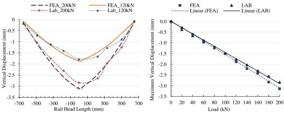
Figure 14. Comparison between Lab and FEA results of the 3-point bend test
