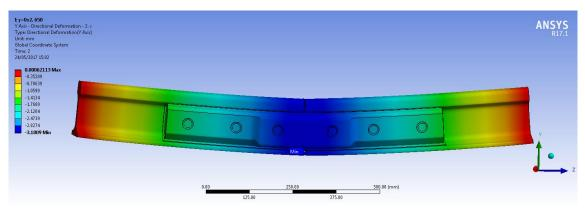
Figure 13. Exaggerated deformed deflection shape of the 3-point bend FE model
