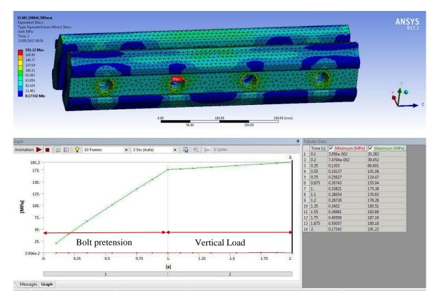
Figure 4.37 Equivalent (Von Mises) stresses-Mecanical-4H-100kN preload-Load case 2
