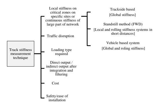
Figure 2.7 Factors affecting track stiffness measurement technique
