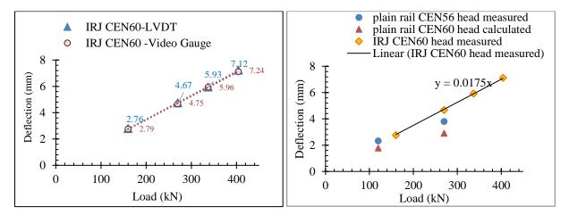
Figure 4.3 (i)Validation of VG deflection data against LVDT deflection data and (ii) Comparison between plain rail and IRJ deflection data measured by the VG.
