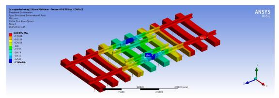
Figure 8. Deformation of suspended IRJ enhanced with strap rails (SR SUS-IRJ) with 30 kN/mm support stiffness per sleeper end.
