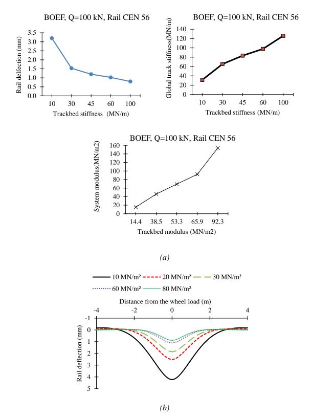
Figure 1. Results from BOEF for (a) various trackbed stiffness and (b) various support system moduli
