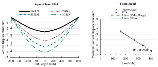
Figure 18. Comparison between FEA data and lab results for the 4-point bend test.
