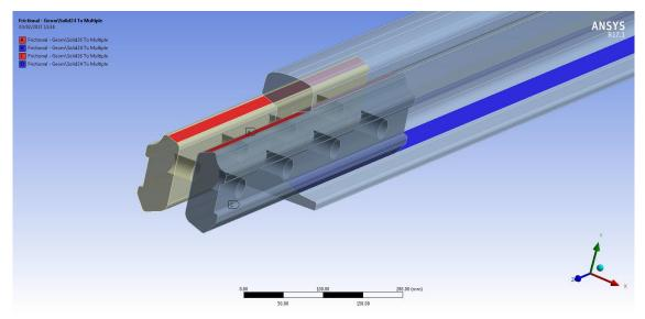
Figure 7. Frictional contact between rail and standard fishplate.
