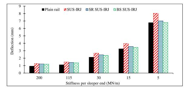
Figure 10. Effect of reinforcement on displacement of suspended IRJ for varying support stiffness
