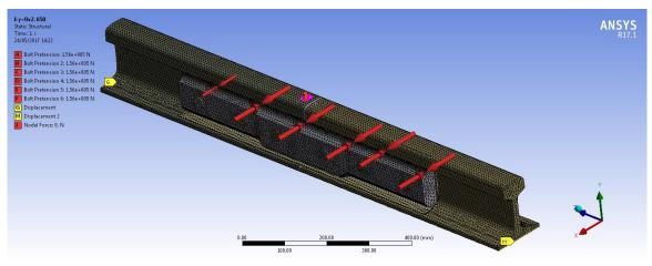
Figure 12. Mesh and boundary conditions of the 3-point bend FE model
