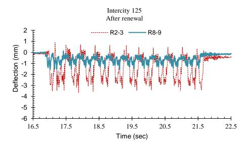
Figure 4. Examples of time –deflection plots of rail web positions in the transition zone under the same passage of Intercity 125.
