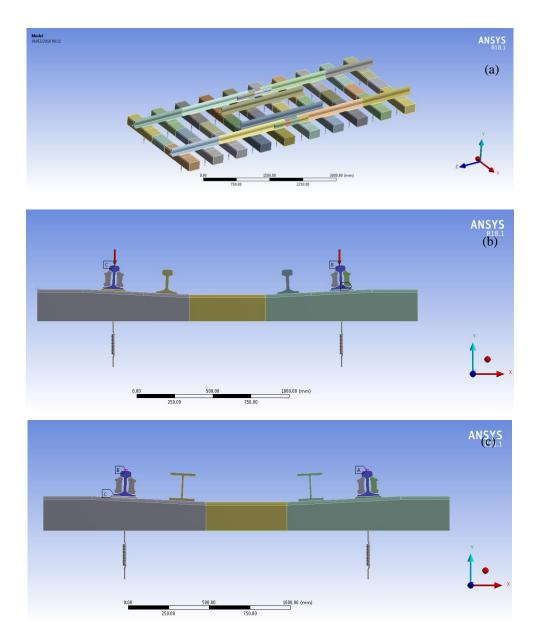
Figure 4.22 View of the Suspended IRJ model enhanced with (a, b) strap rails and (c) I-beams of same length as in (a) from Paper 2
