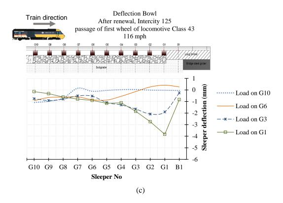
Figure 7. Deflection bowl of the transition zone (a) prior to renewal due to Class 222 first wheel passage and (b) prior to renewal due to Class 43 and (c) after renewal due to Class 43.
