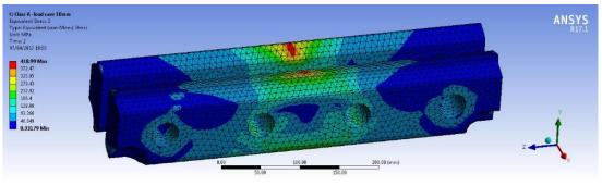
Figure 20. Equivalent (von Mises) stresses - Glued Class A IRJ
