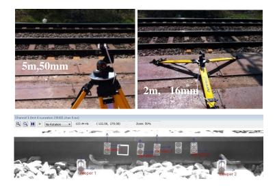
Figure 4.4 View of set-up at site A and video image of single camera showing target array in rail and sleepers.
