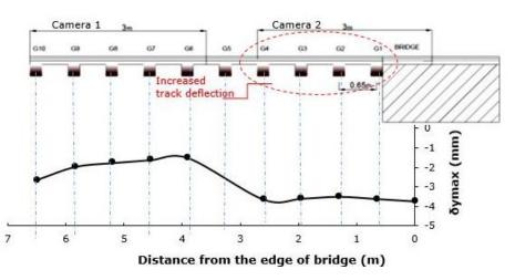
Figure 6. Transition zone general layout and maximum sleeper dynamic displacements at the approach of an overbridge
