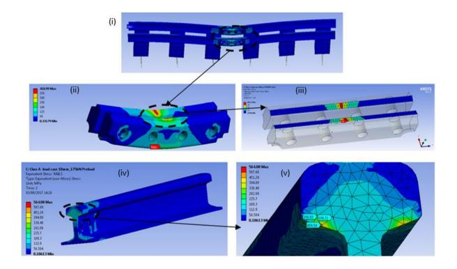
Figure 4.31 Example for glued Class A IRJ –load case 1 (i) deflection (exaggerated in scale) (ii)von-Mises stress at fishplates in average <190 MPa, (iii)von Mises stress at fishplate top fishing surfaces (iv, v) stress singularity in rail end head-web fillet area
