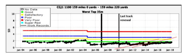
Figure 4.12 CCQ chart-SD values for vertical alignment for Site B.
