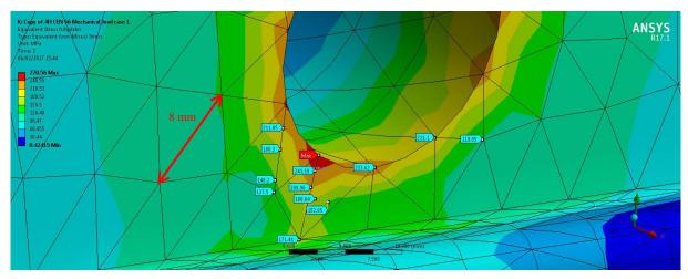
Figure 4.33 Peak von Mises stress in the fishplate hole, 270 MPa, decreased to 150 MPa in 4 mm radius - Mechanical RJ- Load case 2
