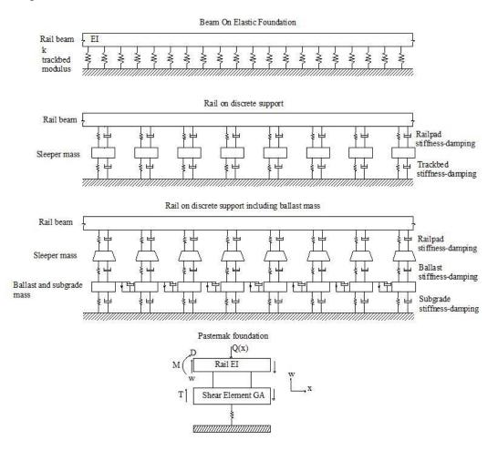
Figure 2.4 Models of rail-track system idealisation produced according to Feng (2011)
