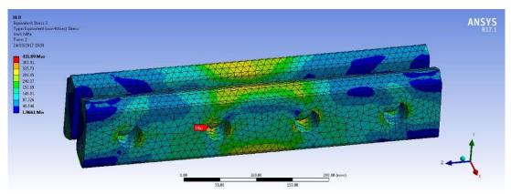
Figure 23. Equivalent (von- Mises) stresses - Dry Class C IRJ
