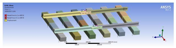
Figure 4. View of the model showing the loading positions at 10mm from the rail end.
