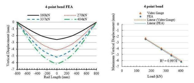
Figure 4.40 Comparison between FEA calculated and VG measured deflection results for the 4-point bend test
