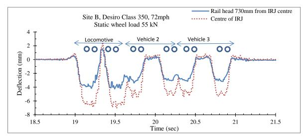
Figure 4.9 Deflection time history under the passage of three-vehicle Desiro at 72mph.
