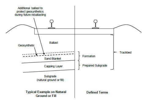
Figure 1.2 Trackbed components according to Network Rail (2016)
