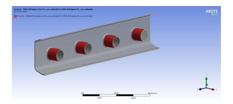
Figure 9. Frictional contact between (a) rail and liner top and bottom fishing surfaces, (b) liner and fishplate and (c) faces of insulated ferrules (incorporated with the liner) to that of the fishplate.
