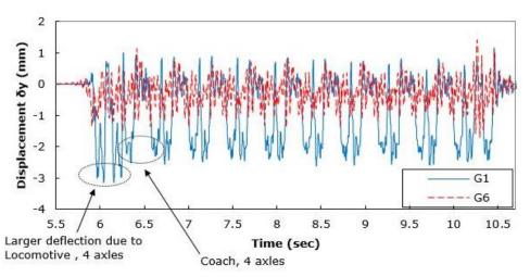
Figure 5. Time- displacement history for the first (G1) and sixth (G6) sleeper in advance of the bridge during Intercity train passage at 125 mph
