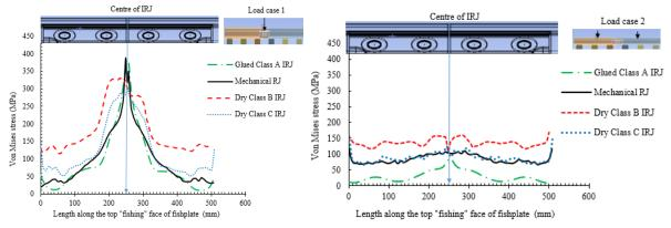
Figure 2. Equivalent (von-Mises) stress plots of the centre of top fishing surface of the fishplate for four rail joint types and two load cases.
