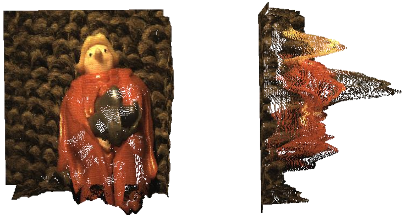
Figure 7.22 Disparity estimation of Lytro data after calibration, illustrated using 3D mesh using MeshLab software
