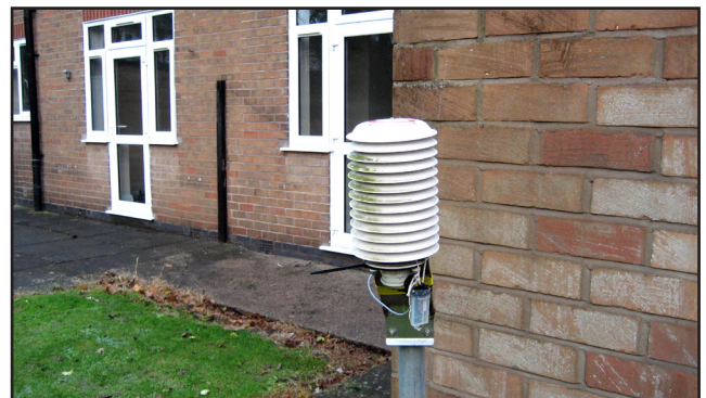
Figure 19. Naturally-aspirated radiation shield for external air temperature monitoring.
