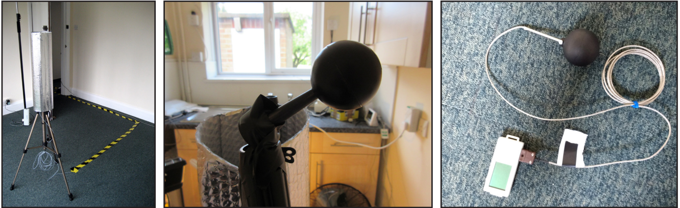
Figure 16. Left – shielded tripod covering wired U-type thermistor. Middle – 40 mm black globe on a U-type thermistor taped to a tripod. Right – battery powered T-type thermocouple.
