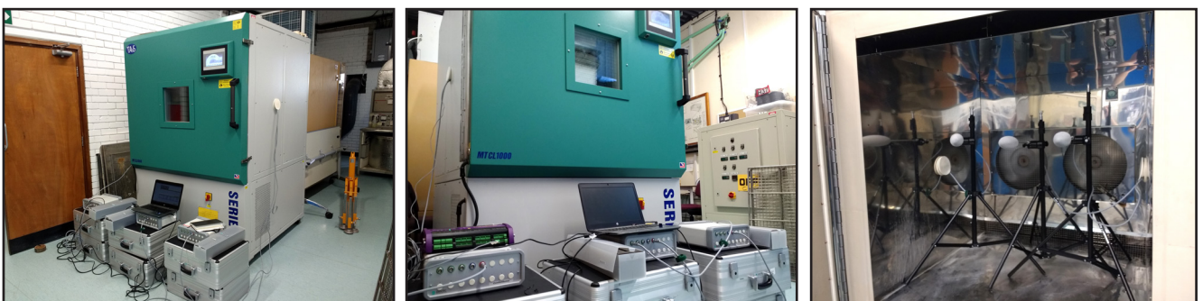
Figure 18. Calibrating operative probes in a climate chamber using a previously calibrated U-type thermistor.
