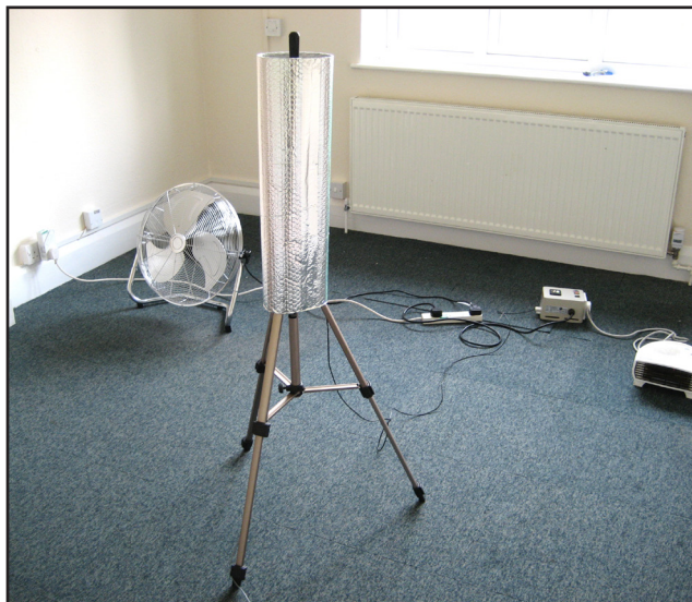
Figure 6. Co-heating equipment deployed in each room.
