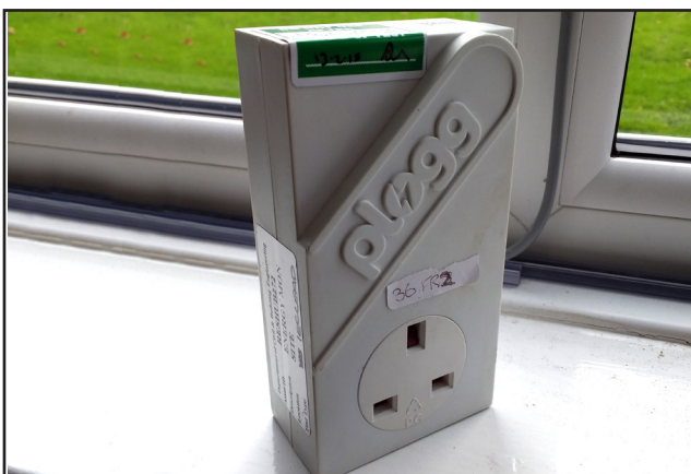
Figure 14. Electricity meter logger plug.
