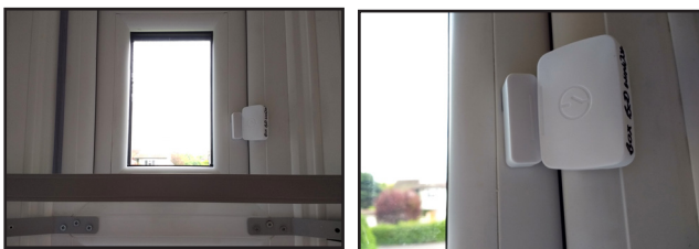
Figure 13. Contact sensor recording window opening.
