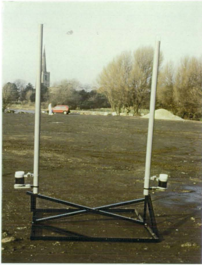
Plate 2.1. The 'tub' traps and supporting apparatus.
