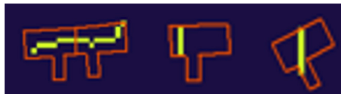
Figure 3. Results of Canny edge detector applied to identify roof ridges on small Nottingham homes.
