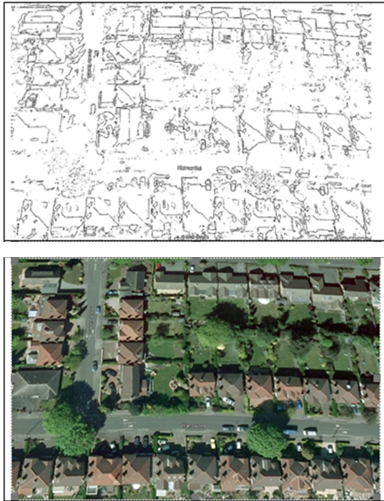
Figure 6. Laplace (weighted high pass) filter with 10 pixel blur applied to a Google Earth image of a residential area in Nottingham.
