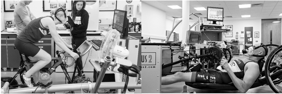
Figure 3.1: Examples of a cycling graded exercise test using road bike (left) or handcycle (right) and the Cyclus 2 ergometer.
