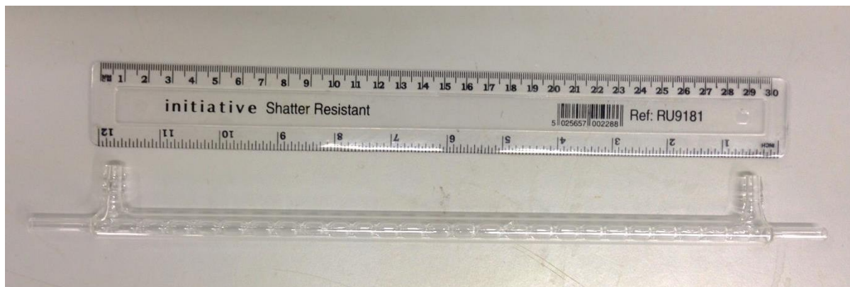
Figure 2.11 SPC design of the mesoscale continuous oscillatory flow crystalliser. SPC meso-tube shown is 30 cm long and has a 5 mm internal diameter.
