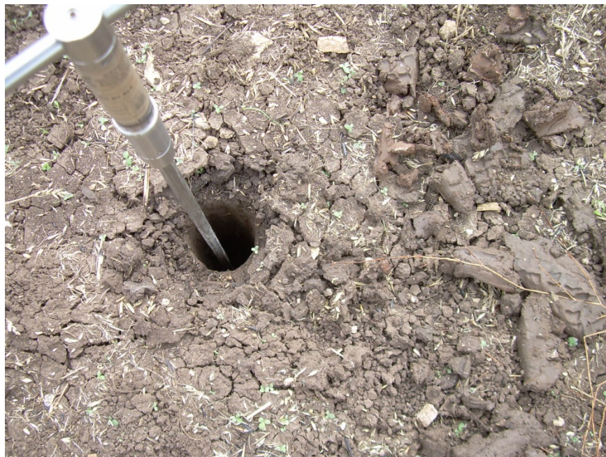
Figure 4.7 – In-situ test with a shear vane for determining soil cohesion (see picture 4.6).
