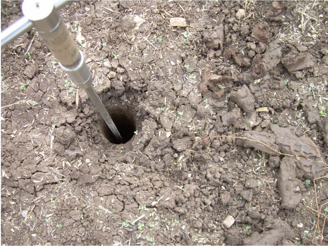
Figure 4.7 (Chapter 4) – In-situ test with a shear vane for determining soil cohesion (see picture 4.6). This picture was taken October of 2012. (See page 95 of this thesis).
