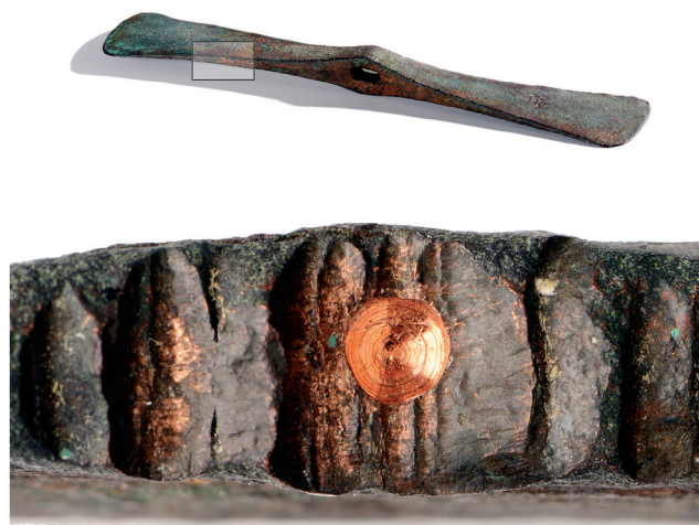
Figure 14 The Escharen double axe with damages for inspecting the composition, and to get a sample (photo National Museum of Antiquities RMO, Leiden)
