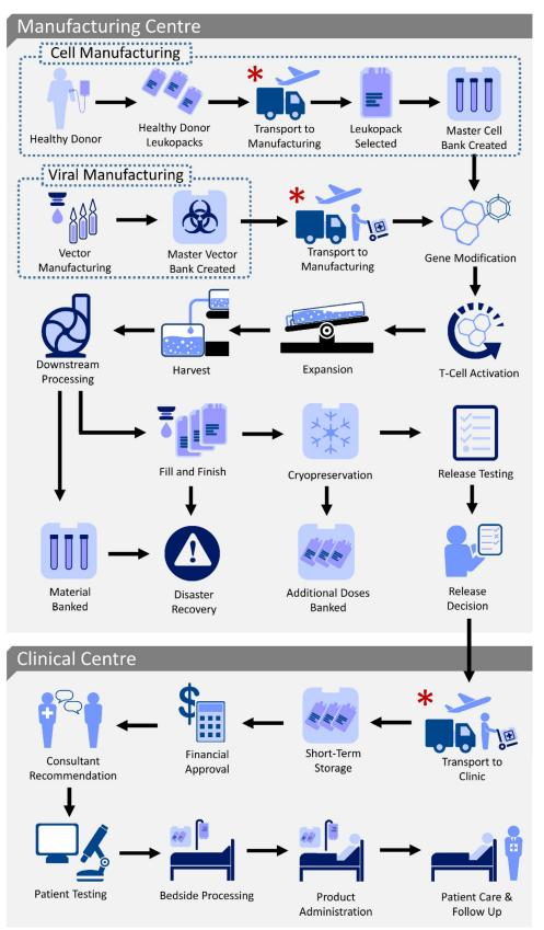
Figure 2. Process flow diagram for manufacturing of allogeneic CAR-T cellular therapies. Items in the dotted-line box are obtained from inventory rather than produced routinely as part of the process. Transport steps are highlighted (red asterisk); inbound clinical products are modelled as originating in the USA with outbound clinical products scheduled for delivery to clinical locations in each country.
