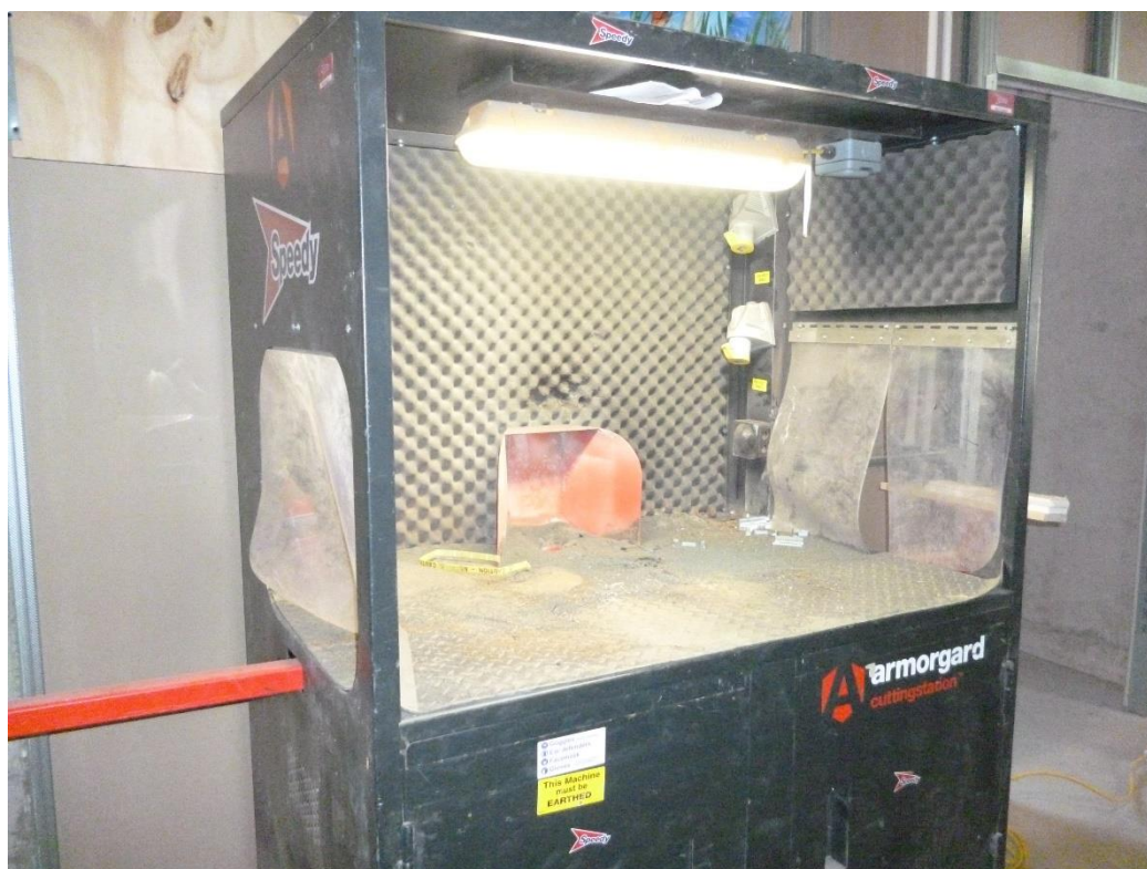
Figure 4 Cutting stations can reduce noise and dust exposures to colleagues working nearby
