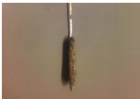
Figure 2.4 Platinum counter electrode used in the research.
