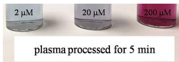
Figure 5.2. Colloidal gold nanoparticles (AuNPs) in poly(3,4-ethylenedioxythiophene) polystyrene sulfonate (PEDOT:PSS) aqueous solutions after synthesis by plasma processing.
