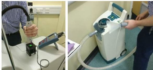
Figure 1. Current laser handpiece with standoff, and separate extraction and collection nozzle.
