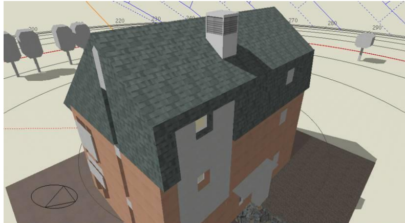
Figure 5-14- Extract from the dynamic model indicating the windcatcher drawing
