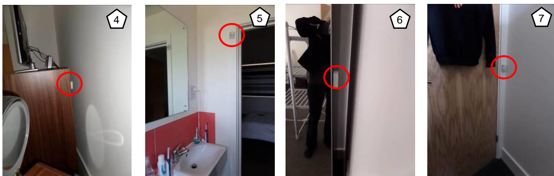
Figure 3-45- Temperature & RH data logger – From left to right - located behind the shaving units in the main bedroom, on the door frame higher than the 1m in the master bathroom, behind the cupboard in bedroom 5 and on the door frame in the drying room where the hot water cylinder is placed (source: author)
