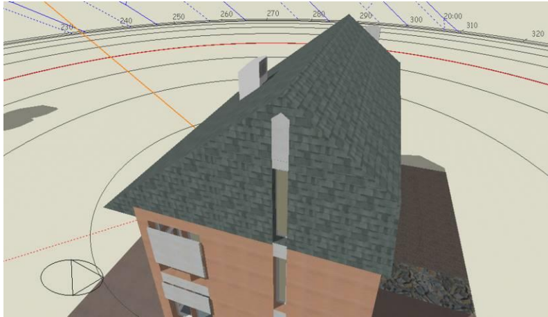
Figure 5-21- Extract from the dynamic model indicating the windcatcher amended design
