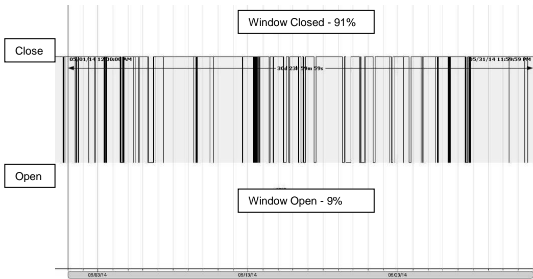
Monitored window operation - D7 - May 2014
