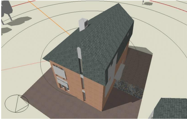
Figure 5-19- Extract from the dynamic model indicating the windcatcher vent located on north side only
