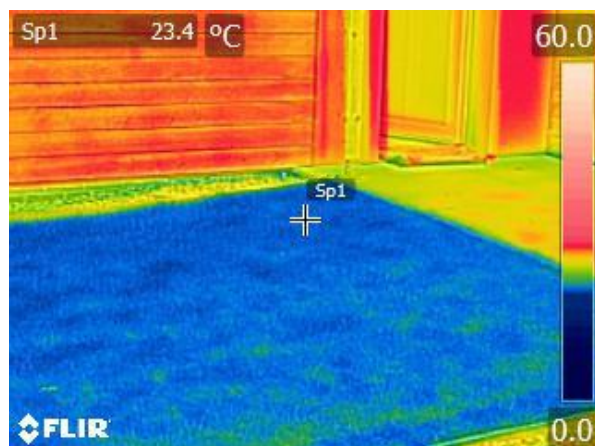
Figure 4-55- Grass temperature of 23.4°C on the ground measured at 3:00pm
