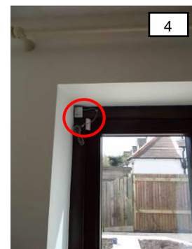
Figure 3-57- State logger & window sensor – From left to right - located on the tilt & turn window in living room, patio door in living room and patio door in dining room (source: author)
