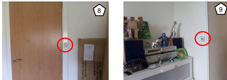
Figure 3-50- Temperature & RH data logger – From left to right - located on the door frame in bedroom 3 and bedroom 4 (source: author)
