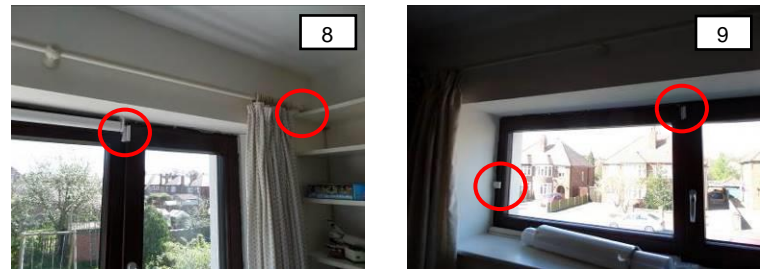
Figure 3-64- State logger & window sensor located on the tilt & turn window in bedroom 5 and bedroom 2 (source: author)
