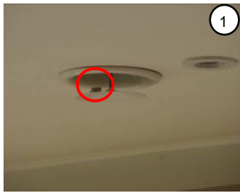
Figure 3-41- Temperature data logger located in the fresh air outlet in the living room (source: author)
