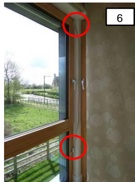
Figure 3-48- State logger & window sensor - From left to right - located on the tilt & turn window in the main bedroom, bedroom and master bathroom (source: author)
