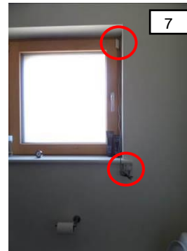
Figure 3-48- State logger & window sensor - From left to right - located on the tilt & turn window in the main bedroom, bedroom and master bathroom (source: author)
