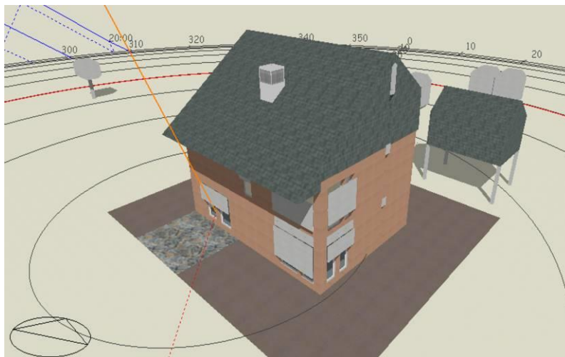
Figure 5-17- Extract from the dynamic model indicating the windcatcher location
