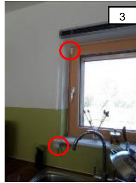
Figure 3-43- State logger & window sensor - From left to right located on the tilt & slide window in the dining room, living room, kitchen and study area (source: author)
