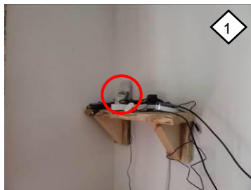
Figure 3-55- CO 2 logger located on the shelf in the living room (source: author)
