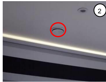
Figure 3-47- Temperature data logger located in the fresh air outlet in the main bedroom (source: author)
