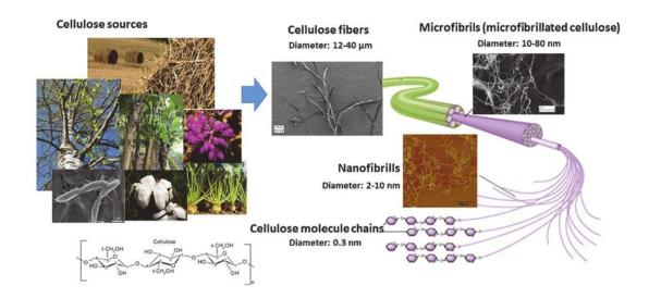
**Figure 2.1.** Different sources from where cellulose can be extracted, including plants, cotton and bacteria. Microscopic morphology of cellulose fibres, microfibrils and nanofibrils, with their schematic representation at molecular level (from alvenotes.com and [59]).
