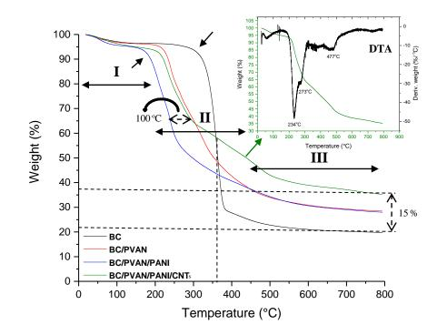
**Figure 7.10.** Thermogravimetric curves of BC nanocomposites characterized by three weight loss stages accordingly marked as I, II and III. The differential thermal curve of BC/PVAN/PANI/CNTs (DTA) is also shown.
