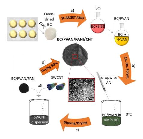
**Figure 7.1.** Schematic diagram of step-by-step reaction of BC modification for synthesis of BC/PVAN/PANI/CNTs nanocomposites. a) SI-ATRP of 4-VAN onto BC, starting with the creation of initiating sites on OH-rich BC surface (BCi) with BiBB. b) COP of ANI performed in an ice-bath in 1M HCl solution and APS as oxidant, to obtain BC/PVAN/PANI. c) Five-time dipping and drying process in SWCNTs dispersion for CNTs-reinforcement forming BC/PVAN/PANI composites.
