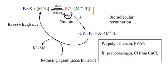
Figure 3.4. Mechanism of metal complex-mediated ARGET ATRP.
