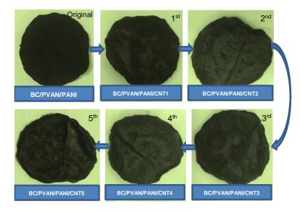
**Figure 7.2.** Optical images of BC/PVAN/PANI membranes after dipping/drying process in CNTs solution continuously performed 5 times. The numeral index (1...5) indicates the dip times in CNTs.
