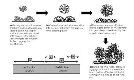
**Figure 2.12.** Schematic diagram of the self-assembling mechanism of PANI into 3D granular structures [98].
