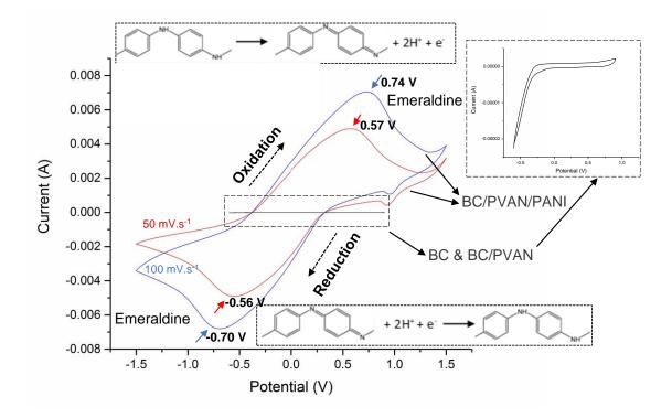
**Figure 6.4.** Cyclic voltammogram curves of BC, BC/PVAN and BC/PVAN/PANI recorded at 50 and 100 mV.s<sup>-1</sup> of scan rates, with the respective magnification of BC and BC/PVAN curves, showing the oxidation and reduction processes of PANI. Red and blue arrows point out to the peak currents corresponding to emeraldine (EM) measured at 50 and 100 mV.s<sup>-1</sup>, respectively.
