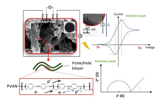
**Figure 6.1.** Schematic representation of the electrical and electrochemical conduction in PVAN/PANI coated BC nanofibrous membranes.
