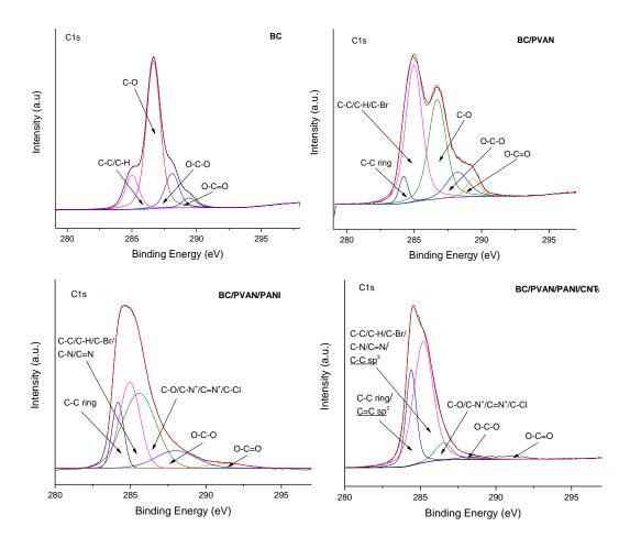
**Figure 7.7.** High-resolution core-level spectra of C1s of BC, BC/PVAN, BC/PVAN/PANI and BC/PVAN/PANI/CNTs nanocomposites, extracted from XPS wide scans of Figure 7.6. Highlighted are the contributions of CNTs to BC/PVAN/PANI/CNTs nanocomposites.
