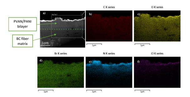
**Figure 5.4.** a) STEM image showing the microstructure of PVAN/PANI-grafted BC at a cross sectional view, as illustrated in Figure 5.2g-h. b-f) corresponding EDX maps of the selected area in a) (Reproduced by permission from Carbohydr Polym, Elsevier, [188] copyright 2019).
