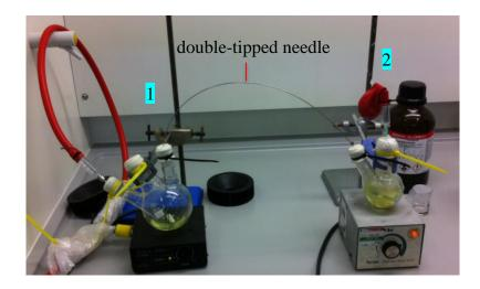
**Figure 3.8.** ATRP reaction of VAN after inserting ASCA conducted under argon atmosphere. **1**, VAN, CuCl<sub>2</sub>, PMEDTA and ASCA dissolved in DMF. **2**, BCi membranes in DMF. Solution 1 is being transferred to solution 2 through the double-tipped needle connecting both flasks.
