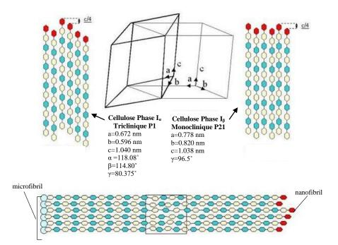
**Figure 2.4.** Crystal form of cellulose type I found in BC, with a schematic representation of the coexisting allomorphisms,  $I_{\alpha}$  and  $I_{\beta}$  crystal units, within the same microfibril. Disorganisation of the microfibrils can occur (amorphous area), as marked in the squared area (adapted from [67]).
