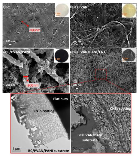
**Figure 7.3.** SEM images of a) pristine BC, b) BC/PVAN, c) BC/PVAN/PANI and d) BC/PVAN/PANI/CNTs, membranes with e) and f) STEM images of a CNTs coating portion of BC/PVAN/PANI/CNTs accordingly identified. The pictures placed on the right corner in SEM images correspond to the respective nanocomposites. The circle area indicates PANI-nanorods.
