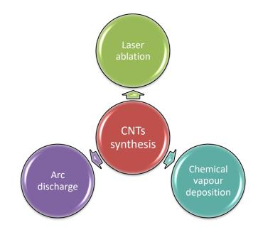
Figure 2.24. Common methods used for CNTs synthesis.
