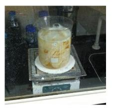
Figure A.2. BC membranes in a boiled NaOH solution.
