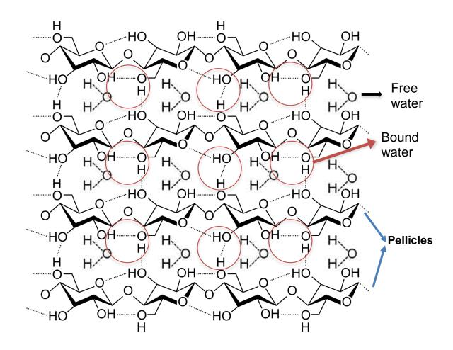
Figure 4.9. Schematic of the molecular structure of BC and their bound and free water [169].
