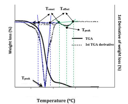
**Figure 3.16.** Illustrative TGA and 1st derivative TGA curves, showing the onset ( $T_{onset}$ ), offset ( $T_{offdset}$ ) and peak temperatures ( $T_{peak}$ ) extrapolated from the first derivative curve (adapted from [168]).
