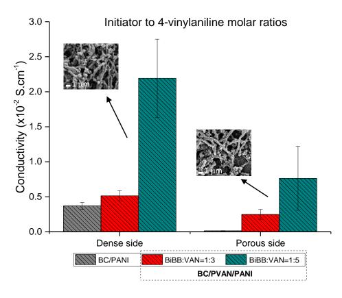
**Figure 6.2.** Electrical conductivity of BC/PANI, and BC/PVAN/PANI membranes with different BC to VAN molar ratios, the embedded images show the morphology of the selected area.(Reproduced by permission from Carbohydr Polym, Elsevier, [188] copyright 2019).
