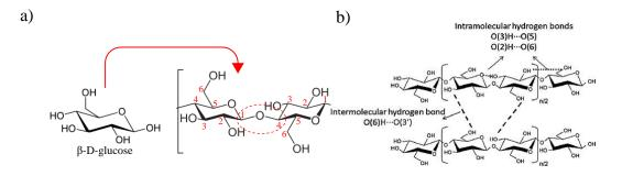
**Figure 2.2.** Chemical structure of (bacterial) cellulose. a) Molecular structure of cellulose repeating unit, cellobiose, showing the  $\beta$ -1,4 linkage between the two D-glucose units. b) Supramolecular structure with intra- and intermolecular hydrogen bonds stablished between adjacent cellobiose units and other cellulose chains, as well as within the repeating unit (Reproduced by permission from Carbohydr Polym, Elsevier, Vol. 133, [63] Copyrights 2015)
