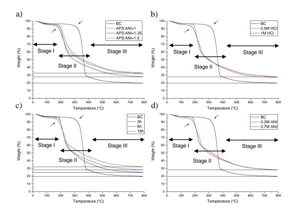
**Figure 5.10.** Thermogravimetric curves of BC/PVAN/PANI 1:5 for different aniline polymerisation parameters. a) aniline concentration, b) oxidant to aniline molar ration, c) reaction time and d) acid concentration. Three main stages of weight loss identified: Stages I, II and III.
