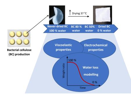
**Figure 4.1.** Schematic diagram illustrating BC membranes subjected to dehydration at 37 °C, with water loss modelling aiming the prediction of the viscoelastic and electrochemical properties of BC membranes.
