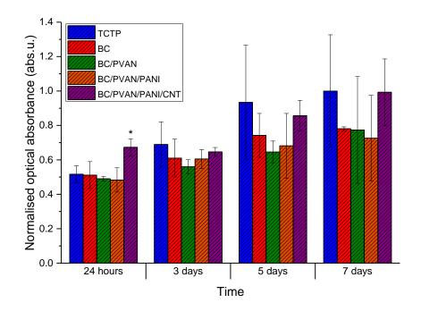
**Figure 8.4.** Cell activity of PC-12 Adh cells cultured on pristine BC, BC/PVAN (at 1:3 and 1:5) and BC/PVAN/PANI (at 1:3 and 1:5). The results are shown in terms of means $\pm$ standard deviations of optical absorbances measured. \* indicates statistical significance (p<0.05) compared to TCTP and BC according to one-way ANOVA testing.
