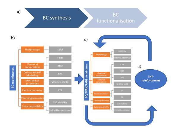
**Figure 3.1.** Schematic diagram of the processes involved in the production and characterisation of pristine BC and BC nanocomposites accordingly described in Chapter 3. a) Synthetic procedure of BC membranes followed by their functionalisation, and b-d) corresponding characterisation methods used.
