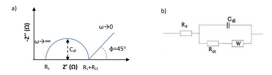
**Figure 3.15.** a) Example of Nyquist plot with a diffusion line obtained from the equivalent Randles circuit shown in b).  $R_s$ ,  $R_{ct}$ ,  $C_{dl}$  an W stands for solution resistance, charge transfer resistance, double layer capacitance and Warburg impedance.
