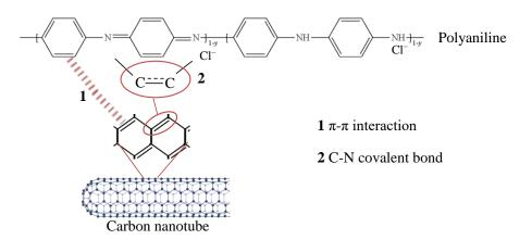
**Figure 7.11.** Schematic illustration of the possible interactions stablished between PANI and CNTs. 1 shows the pi-stacking interaction between the aromatic rings of both PANI and CNT and in 2, CNTs competes with chloride (Cl<sup>-</sup>) to dope PANI and form a covalent C-N bond (adapted from [80]).
