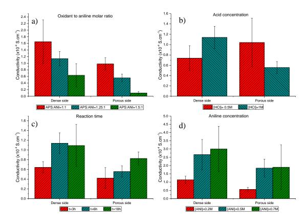
**Figure 6.3.** Differences on the electrical conductivity of BC/PVAN/PANI composites with variation of aniline polymerisation parameters: a) molar ratio APS:ANI, b) acid concentration, c) reaction time and d) aniline concentration (Reproduced by permission from Carbohydr Polym, Elsevier, [188] copyright 2019).
