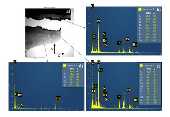
**Figure 5.5.** TEM-EDX map sum spectra of BC/PVAN/PANI in three different regions/levels of the membrane indicated in a), which correspond to the area shown in Figure 5.2h. b-c) surface coatings of PVAN/PANI as represented in Figure 5.2hi and d) BC substrate as represented in Figure 5.2hj.
