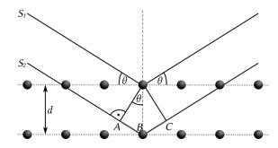
**Figure 3.11.** Schematic representation of the XRD in a crystalline structure, according Bragg's law. Incident X-rays (S<sub>1</sub> and S<sub>2</sub>) reach the parallel planes of ions d-spaced, that are reflected at an angle  $\theta$ , the same as the incident angle.
