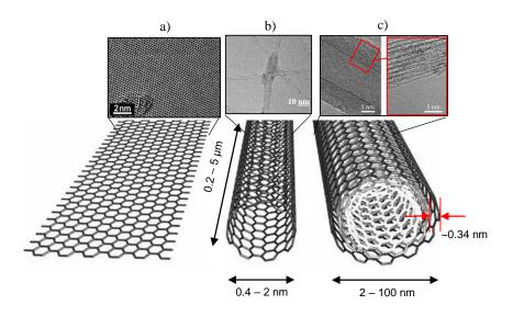
**Figure 2.21.** Molecular structure of a) a graphene sheet, b) SWCNTs and c) MWCNTs [130], and corresponding transmission electron microscopic (TEM) images on the top, showing the single (in SWCNTs) and the multiple walls (in MWCNTs) composing CNTs [131–133].
