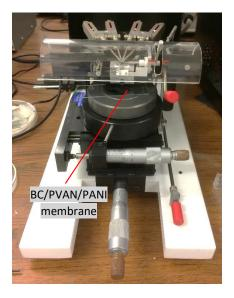
**Figure 3.12.** Jandel four-point probe set-up used to measure the sheet resistance of BC/PVAN/PANI membrane samples.
