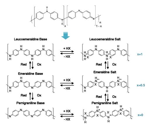
**Figure 2.7.** Different oxidation forms of PANI. The highest conductive form, emeraldine salt, can be reduced to leucoemeraldine salt that is non-conductive, or can be fully oxidised to pernigraniline that is less conductive than emeraldine. These three oxidation states can be further deprotonated into their respective base forms in a reversible manner (adapted from [85]).
