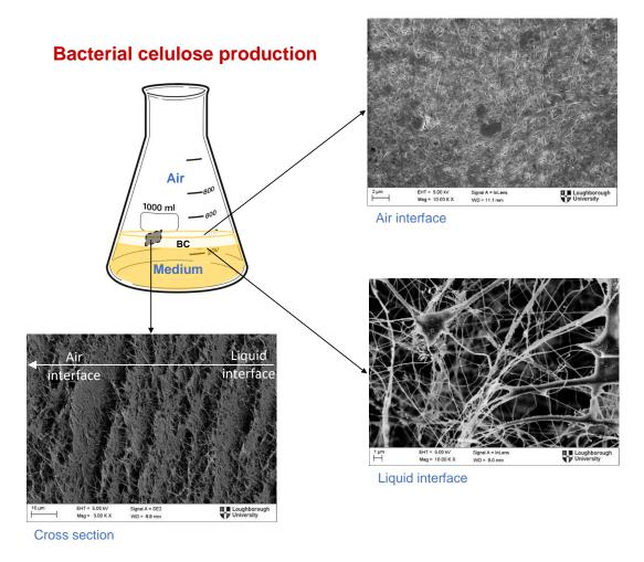
**Figure 4.2.** Diagram of BC production displaying SEM images of both surfaces of a freeze-dried membrane, interfacing air and liquid respectively, and a cross section [169].
