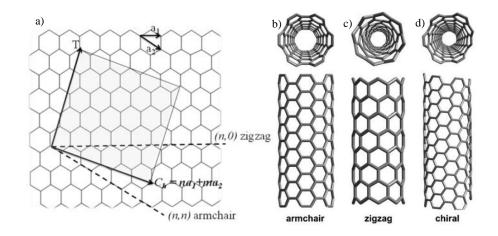
**Figure 2.22.** Molecular representation of the possible atomic configurations of CNTs. a) representation of the vectors corresponding to b) airmchair, c) zigzag, and d) chiral-based conformations [137].
