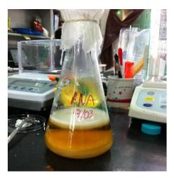
Figure A.1. BC membrane in an Erlenmeyer flask covered with filter paper.
