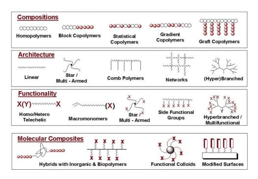
**Figure 2.16.** Examples of possible molecular structures that can be synthesised with ATRP (Reproduced by permission from Mater Today, Elsevier, Vol. 8, Issue 3, [114] Copyrights 2005).
