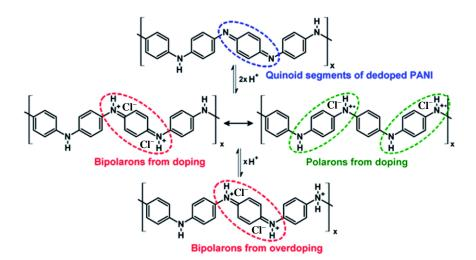
**Figure 2.9.** Doped and dedoped forms of emeraldine oxidation state of PANI, showing the polaron and bipolaron structures after protonation with HCl. The counterions from the dopant ( $Cl^-$  in the present example) compensate the charge carriers introduced after doping.[94].
