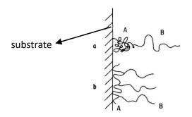
**Figure 2.13.** Examples of polymeric steric stabilisers in the form of a) block copolymers and b) graft copolymers, where A is the polymer with the anchor group and B is the polymer that provides the steric barrier [104].
