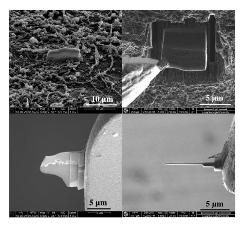
**Figure 3.10**. FIB/SEM images from different perspectives and magnifications illustrating the FIB liftout process used to extract a thin film TEM sample from the bulk membrane sample.
