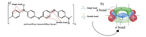
**Figure 2.8.** PANI in the emeraldine base structure. a) Polyconjugated system showing the alternating single and double bonds in the polymer backbone, formed by sigma ( $\sigma$ ) and pi ( $\pi$ ) bonds. b) Schematic representation of  $\sigma$  and  $\pi$  orbitals overlapping each other to form a double bond between two carbon atoms (adapted from [91]).  $\sigma$ -bonds gives the strength to the strain, while  $\pi$ -bonds ensure delocalisation of the electrons.
