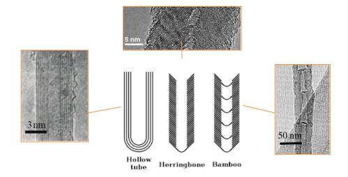
**Figure 2.23.** Examples of coexisting morphologies of MWCNTs: hallow tube, herringbone and bamboo (adapted from [138–140]).
