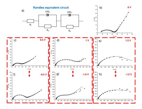
**Figure 6.5.** a) Randles equivalent circuit used to fit the impedance spectra shown in b-h.b-h) Nyquist plots of representative impedance data of BC/PVAN/PANI nanocomposites collected from different applied DC potentials upon superimposition of a sinusoidal AC potential of 10 mV. The solid lines (—) represent the fitting by the circuit in a).
