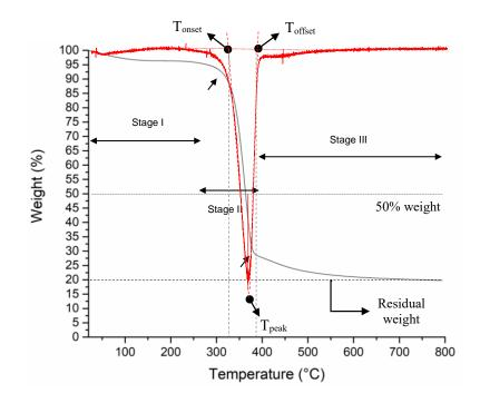
**Figure 4.5.** Representative thermogravimetric curve of 5 BC samples (black) and corresponding first derivative (red) from which the onset ( $T_{onset}$ ), offset ( $T_{offset}$ ) and peak ( $T_{peak}$ ) temperatures were measured. Three main weight loss stages are identified: Stages I, II and III.
