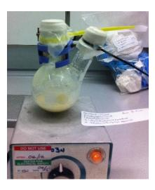
Figure 3.7. Initialisation reaction of BC surface performed with BiBB kept under argon atmosphere.
