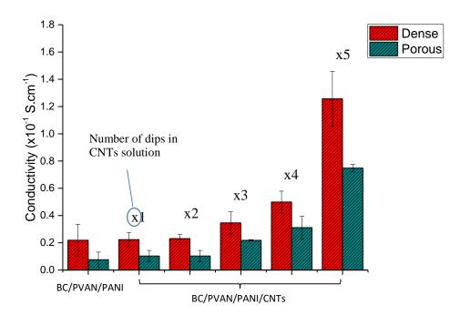
**Figure 7.8.** Electrical conductivity of BC/PVAN/PANI nanocomposites before and after immersion in CNTs dispersion for one up to five times.
