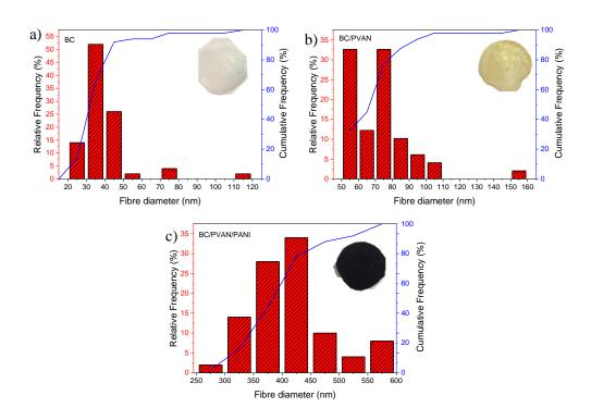
**Figure 5.3.** Histogram of the diameter (relative frequency) of the fibres of a) BC, b) BC/PVAN, and c) BC/PVAN/PANI membranes, showing the respective cumulative frequencies (solid line –).
