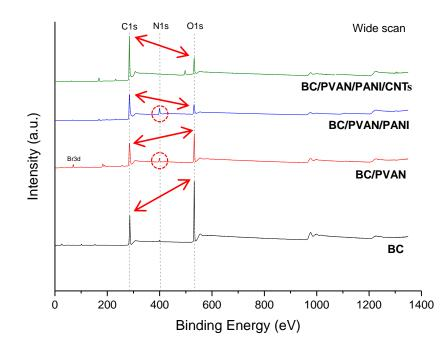
**Figure 7.6.** Comparative XPS spectra of wide scans acquired for un-modified BC, and BC/PVAN, BC/PVAN/PANI and BC/PVAN/PANI/CNTs nanocomposite membranes. The double sized arrows point out to the contrasting peak intensities of C1s and O1s after the inclusion of the successive coatings onto BC, and the circular areas in BC/PVAN and BC/PVAN/PANI spectra identify the peaks ascribed to N1s.
