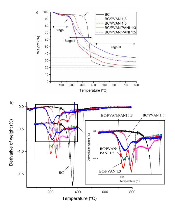
**Figure 5.9.** a) Thermogravimetric curves of BC, BC/PVAN and BC/PVAN/PANI nanocomposites with BiBB:VAN molar ratios of 1:3 and 1:5, measured from room temperature to 800 °C. Three main stages
