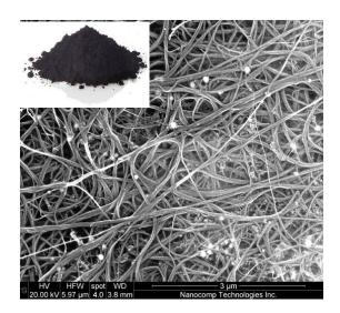
Figure 2.18. SEM [121] and optical [122] images of CNTs powders.
