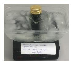
Figure 3.9. COP of aniline performed on BC/PVAN membranes conducted in an ice-bath (~0-5 °C).
