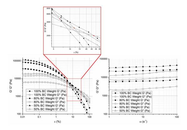
**Figure 4.6.** Representative curves of storage (G') and loss (G'') moduli of BC membranes holding 100, 80 and 50 % water, measured as a function of strain (left) and frequency (right). The red dots indicate the interceptions between G' and G''.[169].
