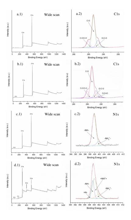
**Figure 5.8.** Typical wide scans of a.1) BC, b.1) BC-BiBB, c.1) BC/PVAN (BiBB:VAN=1:5) and d.1) BC/PVAN/PANI (BiBB:VAN=1:5). High resolution C1s scans of a.2) BC and b.2) BC-BiBB, and high resolution N1s scans of c.1) BC/PVAN (BiBB:VAN=1:5) and d.1) BC/PVAN/PANI (BiBB:VAN=1:5). Peaks were curve-fitted using Thermo Scientific<sup>TM</sup> Avantage Data System. (Reproduced by permission from Carbohydr Polym, Elsevier, [188] copyright 2019).
