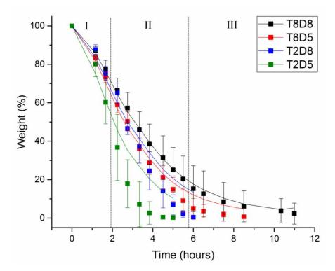
**Figure 4.8.** Experimental water loss (**•**) and respective modelling (—) of BC membranes 8 mm thick and 8 mm of diameter (T8D8), 8 mm thick and 5 mm of diameter (T8D5), 2 mm thick and 8 mm of diameter (T2D8) and 2 mm thick and 5 mm of diameter (T2D5). The water loss curves of each size/thickness correspond to an average of 5 samples and the error bars correspond to the respective standard deviations.[169].
