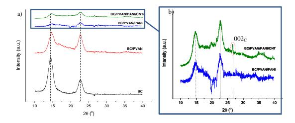
**Figure 7.5.** a) XRD spectra of BC, BC/PVAN, BC/PVAN/PANI and BC/PVAN/PANI/CNTs, b) with the corresponding magnification of the selected squared area. The curves were smoothened with FFT using Origin®2015 software.
