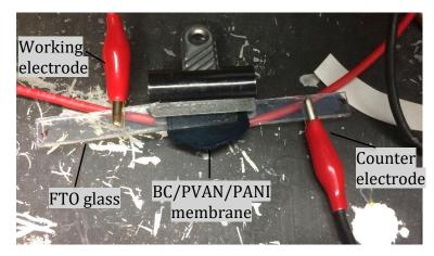
**Figure 3.14.** Illustrative set-up used for electrochemical measurements with a potentiostat. A BC/PVAN/PANI membrane clamped between two pieces of FTO glasses (1 cm per 2 cm).
