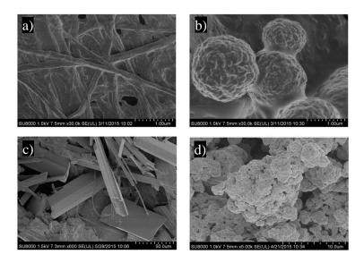
**Figure 2.11.** Examples of 3D and 1D supramolecular structures of PANI that can be obtained: a) Nanofibres, b) granular spheres (granules), c) plates, d) micro-sized granular agglomerates – commercial PANI – (adapted from [97]).
