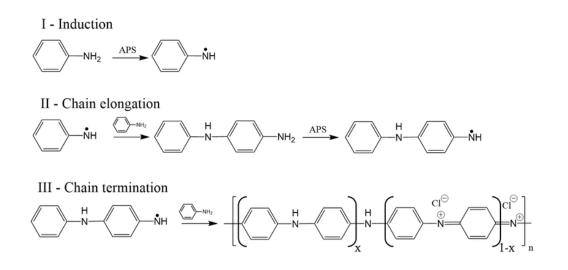
Figure 3.6. Mechanism of aniline polymerisation. I induction, II chain propagation and III chain termination [100].
