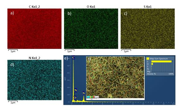
**Figure 7.4.** SEM-EDX of BC/PVAN/PANI/CNTs membranes. a-d) X-ray maps of the selected area f) and e) respective sum map spectrum.
