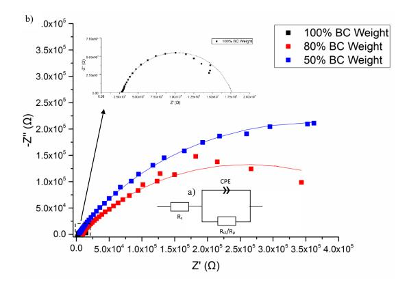
**Figure 4.7.** a) Randles circuit used for fitting the experimental data. b) Representative Nyquist plots of BC membranes with 100% (never-dried membrane), 80 % and 50 % water content. The solid lines (-) represent the respective fittings.[169].
