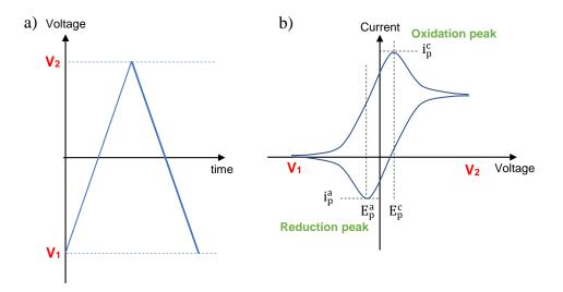
**Figure 3.13.** Schematic representation of a cyclic voltammogram from a single charge-transfer process. a) Applied cyclic excitation signal and b) corresponding response (cyclic voltammogram), showing one oxidation/reduction paired-peak when the potential is swept between V<sub>1</sub> and V<sub>2</sub>.  $i_p^a$  and  $i_p^c$  are the anodic and cathodic peak currents, respectively, and  $E_p^a$  and  $E_p^c$  are the corresponding peak potentials.
