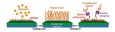
**Figure 2.17.** Schematic illustration of the synthesis of grafted surfaces with ATRP following the 'grafting-from' (left) and 'grafting-to' (right) approaches. In the 'grafting-from', an initiator is attached to the substrate from which polymer chains can grow. In the 'grafting-to', a pre-synthesised macromolecule containing a reactive end group is attached to the substrate that had its surface previously activated.[117].
