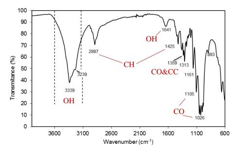
**Figure 4.3.** Representative ATR-FTIR spectrum of BC with indication of the corresponding vibrational modes of the functional groups [169].
