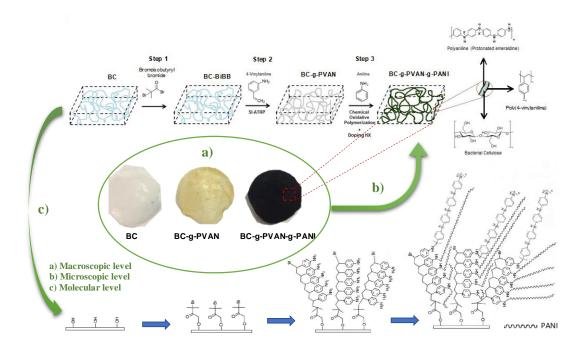
**Figure 5.1.** Schematic synthesis of BC/PVAN/PANI nanocomposite membranes at a) macroscopic, b) microscopic and c) molecular levels. Step 1: Initiator (BiBB) immobilisation onto BC. Step 2: SI-ATRP of 4-VAN onto BC. Step 3: COP of aniline on BC/PVAN in the presence of HCl as doping agent, to form BC/PVAN/PANI. (Reproduced by permission from Carbohydr Polym, Elsevier, [188] copyright 2019).
