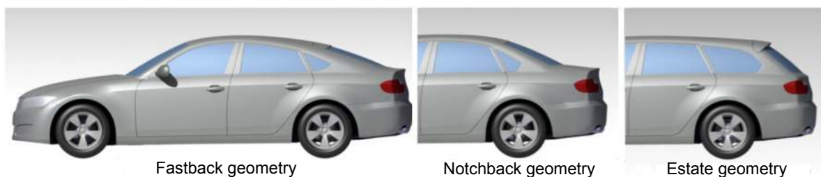
Figure 1.14: Schematic representation of the DrivAer model. Pictures from Heft et al (2012).
