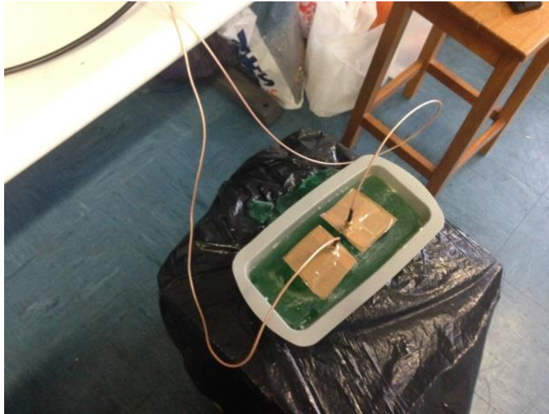
Figure 5.10: Monopoles implanted into the multi-material forearm - radius phantom
