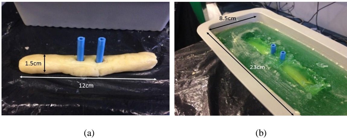
Figure 5.9: a) Bone layer and PLA insulators; b) forearm - radius phantom composed of bone and muscle emulating tissues
