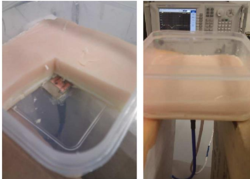
Figure 3.9: A four layer tissue phantom featuring blood, muscle, fat, and wet skin tissue layers for the monitoring of blood glucose levels [59]
