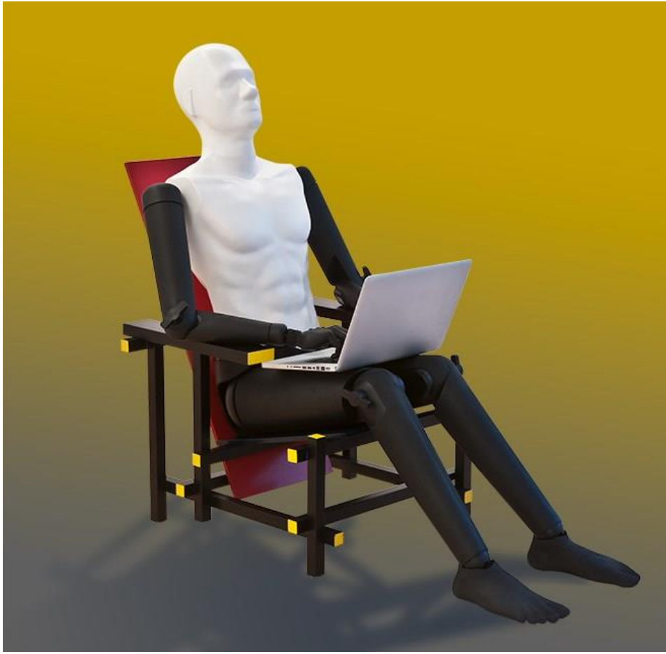
Figure 3.8: An example of realistic shape phantom featuring ceramic (white coloured) and plastic (black coloured) casts [56]
