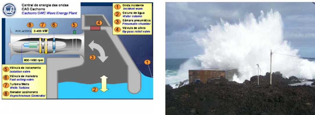
Figure 1.6: The OWC Pico power plant [4], built in 1995 - 1998. The power plant worked for only a short period in October 1999, then was put on standby until 2004. From 2006 the Pico plant was used as a demonstrator and research pilot, with the objective of improving its reliability. In 2010, the plant produced 45 MWh for an operating time of approximately 1,400 h. In 2016, it produced 39 MWh. Nowadays its structure has become weakened and the decision has been made to decommission it [6].
