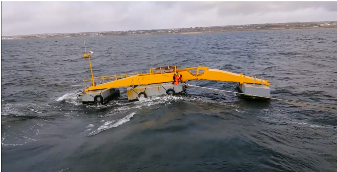
Figure 1.12: The 1/4-scale SeaPower Platform prototype in Ireland [6].
