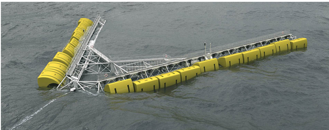
Figure 1.15: WEPTOS wave energy converter is made up of a structure consisting of two adjustable V-shaped arms. Wave energy absorbers of the Salter's Duck type are mounted on each arm [6].
