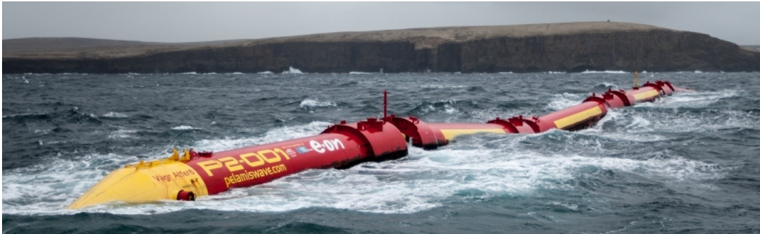
Figure 1.13: The Pelamis P2 operating in Scotland in 2012 [6].
