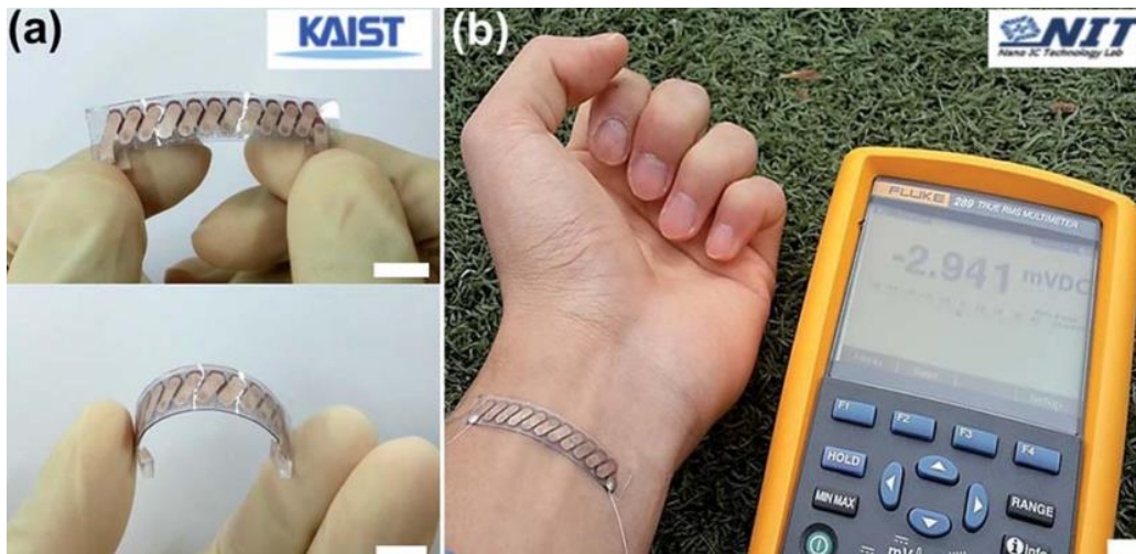
Figure 2-5 Demonstration of band-type flexible TE generator for harvesting thermal energy from human skin: (a) photos of band-type flexible TE generator and (b) electricity generation measured on human skin at an air temperature of 15 °C. Scale bar, 1 cm. [55]
