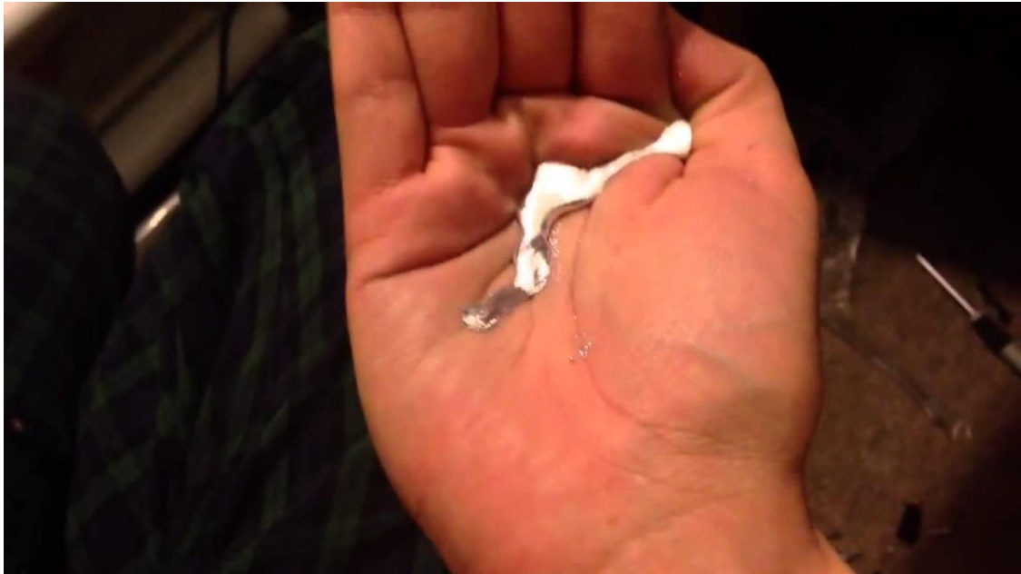
Figure 2-8 Non-toxic Galinstan being handled without protection equipment [97]. This handling has proven to be safe with the only effect being that it can dry out the skin.
