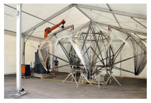
**Figure 2.** Architectural scale prototype of engineered structure demonstrating biomimicry design principle of lobster shell structure using fibrous composite materials assembled through robotic fabrication [57].
