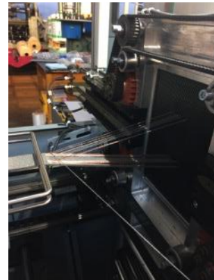
Figures 17. – 18. Weaving process of the conductive strap at TPL's Central Lab (left) and at STFI - Focus Lab (right). © TPL.
