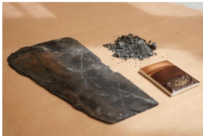
Fig. 3. Rubbles of slate, collected from the worksite of Les Petites Affiches (2018) transformed in pigments and ceramic enamel - © Anna Saint Pierre
