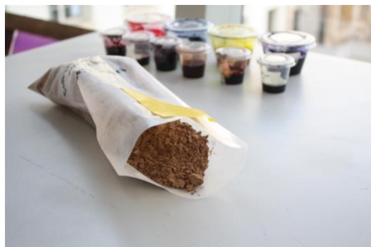
Fig. 14: Pigments produced from the rubbles of bricks incorporated into a screen-printed base.
