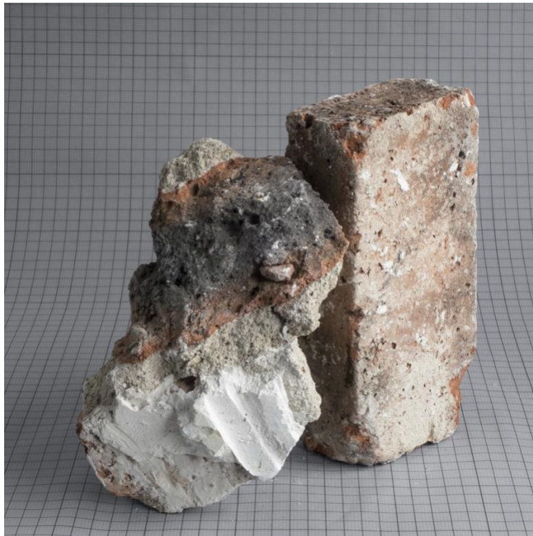
Fig. 11 : Bricks focus - The brick was used on site in filler structured by wire mesh poles. Under the orange shell, their cut-out reveals a colours diversity and intensity : a red to black gradient punctuated by aggregates due to cooking differences and the integration of clinker - industrial waste - in the clay paste. - © Anna Saint Pierre
