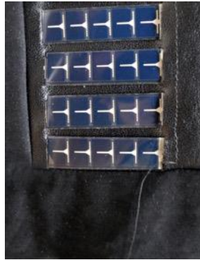
Fig. 7. Solar cells fixated inside leather
