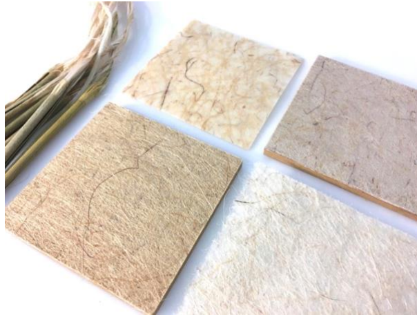
Fig. 3 Muka fibre and prototype Harakeke Nonwoven Materials (top left - Material 3, top right - Material 2, bottom right - Material 1)
