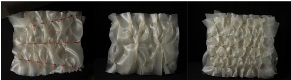
Fig. 4 Variability in three pleated surfaces, differing in number of lines, their orientation, and pleating pattern
