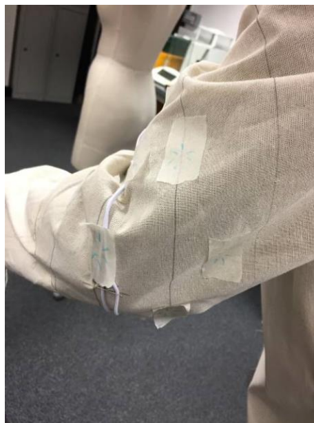
Figure 4: LED positions marked on the toile sleeve using masking tape.
