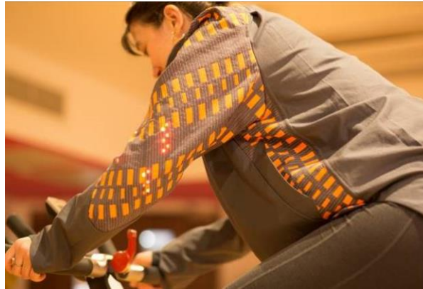
Fig. 1. The woven cycling jacket incorporating LEDs within electronic yarns in the elbows.
