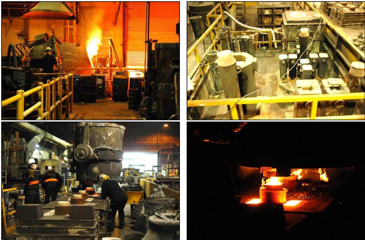
Figure 3.2: A series of photographs showing the manufacturing process and component moulds of the 8 tonne melt manufactured during the IMPACT project.
