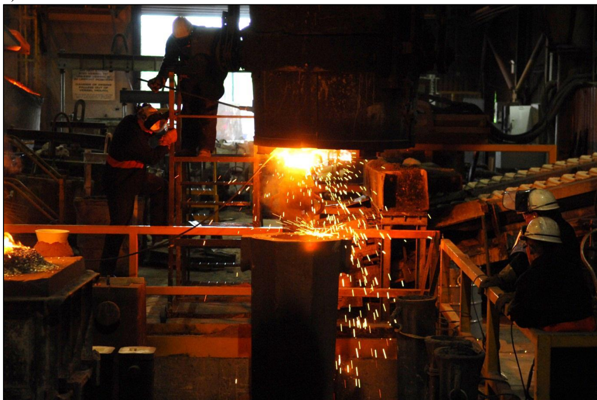
Figure 9.3: Two photographs showing the pouring of the eight tonne melt into the individual moulds.
