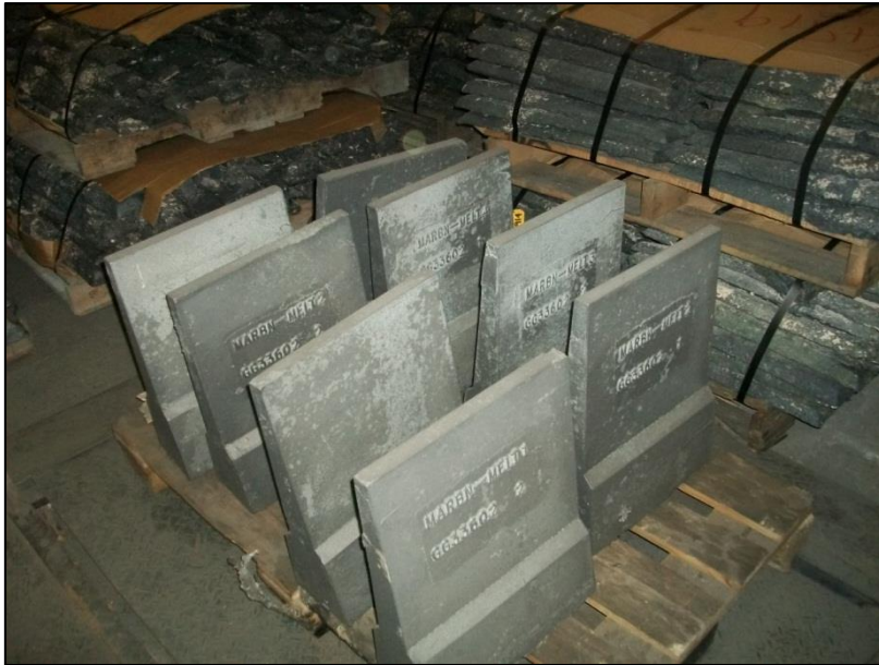
Figure 3.1: A photograph of GAM 1 – 4 plates cast at Goodwin Steel Castings Ltd. Photograph courtesy of R. Leese (Goodwin Steel Castings Ltd).
