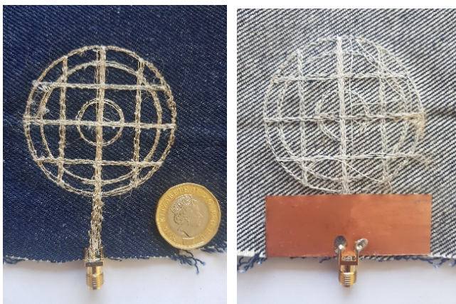
Fig. 14. Embroidered meshed monopole antenna: front and back
