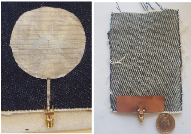
Fig. 5. Fabricated circular monopole antenna: (front and back)
