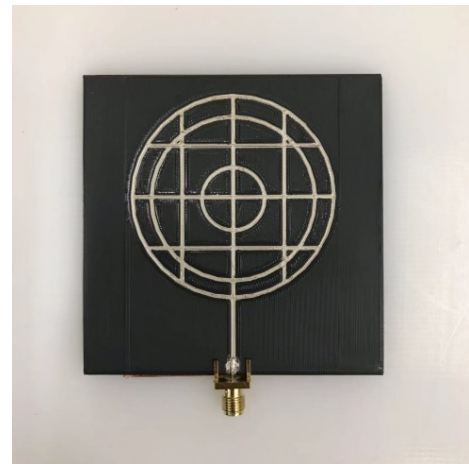
Fig. 17. 3D printed meshed monopole antenna
