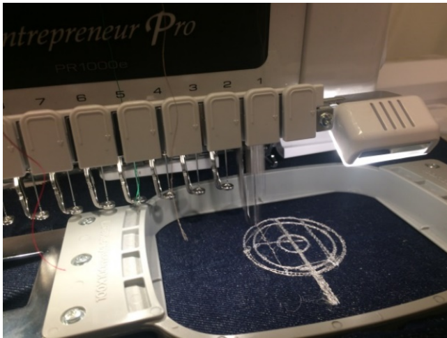
Fig. 13. Meshed monopole being embroidered
