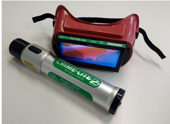
Figure 3 – The green Crime-lite 2 and orange/red filter goggles (OG590) used by participants throughout the study.
