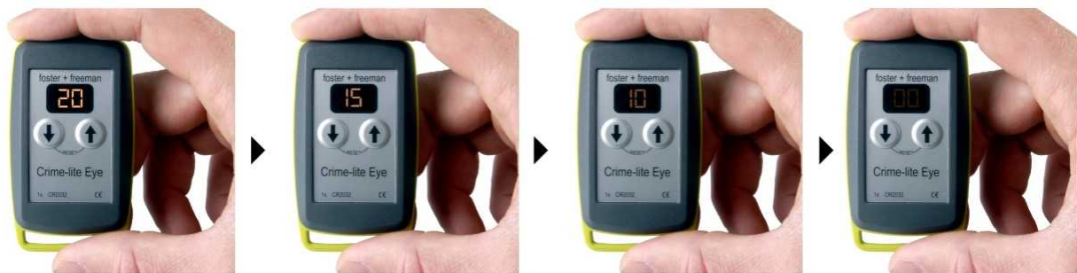
Figure 1 – The Crime-lite Eye™ showing a schematic representation of the dimming display as would be perceived during dark adaptation.
