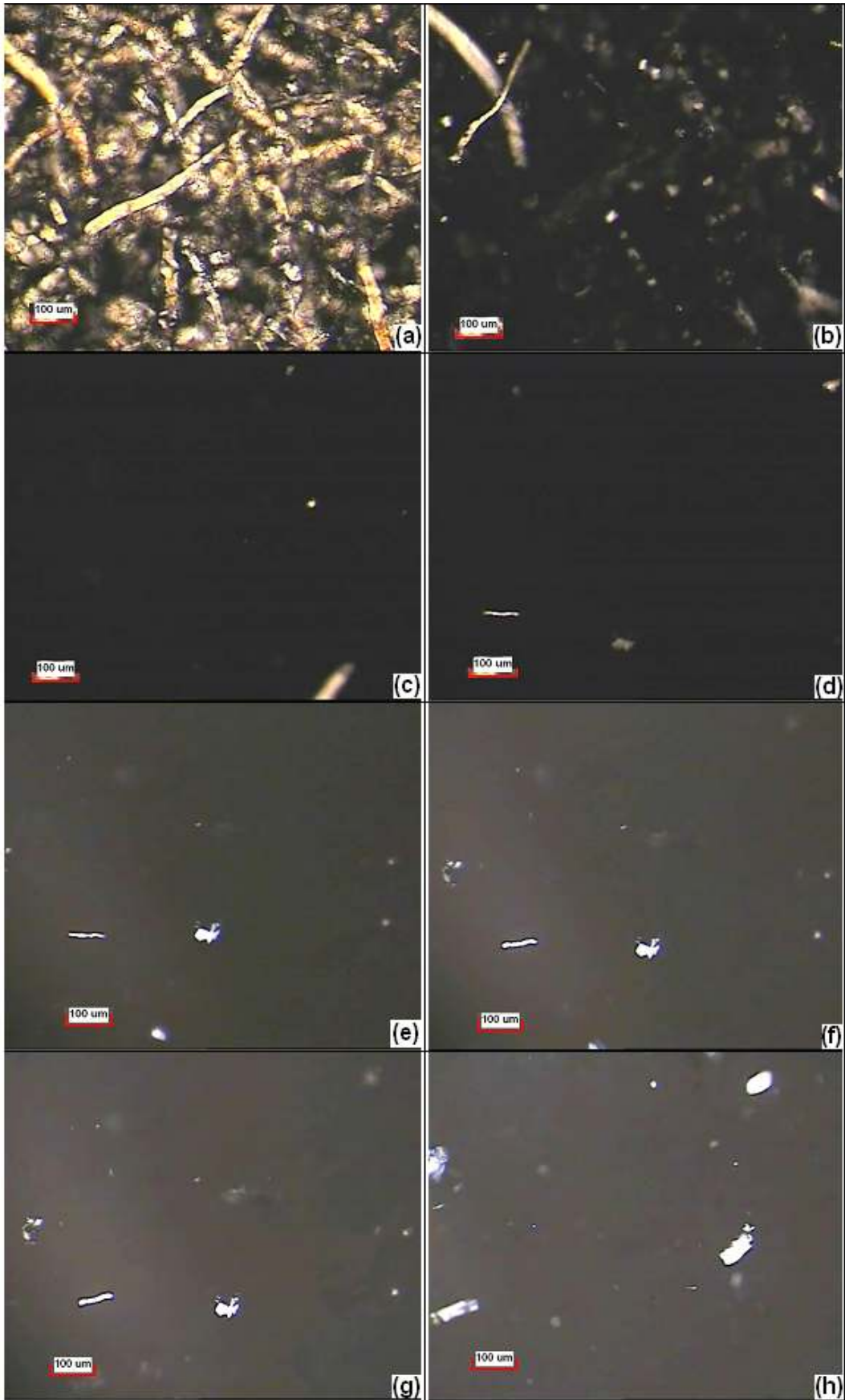
Figure 5-25. 20% MC in propylene glycol during heating at (a) 30 o C (b) 100 o C (c) 120 o C (d) 150 o C, and during cooling at (e) 140 o C (f) 120 o C (g) 100 o C (h) 30 o C
